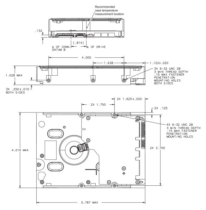
Figure 3. Mounting dimensions (1000 and 750GB models)
