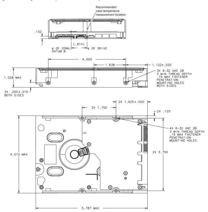
Figure 3 Mounting dimensions (500, 320, 250 and 160GB models)
