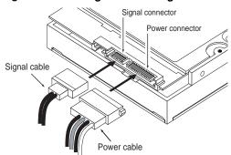
Each cable is keyed to ensure correct orientation. Barracuda drives support latching SATA connectors.
