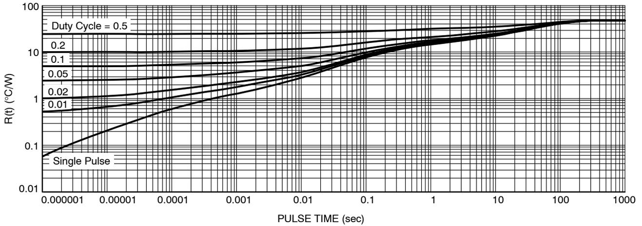
**Figure 13. Thermal Characteristics**
