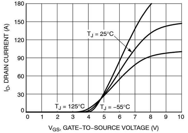
Figure 2. Transfer Characteristics
