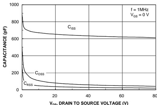
Figure 8. Capacitance Characteristics.
