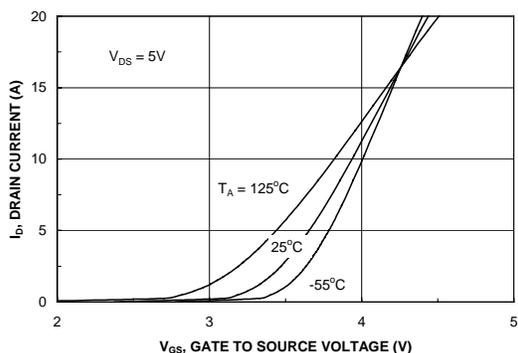
Figure 5. Transfer Characteristics.
