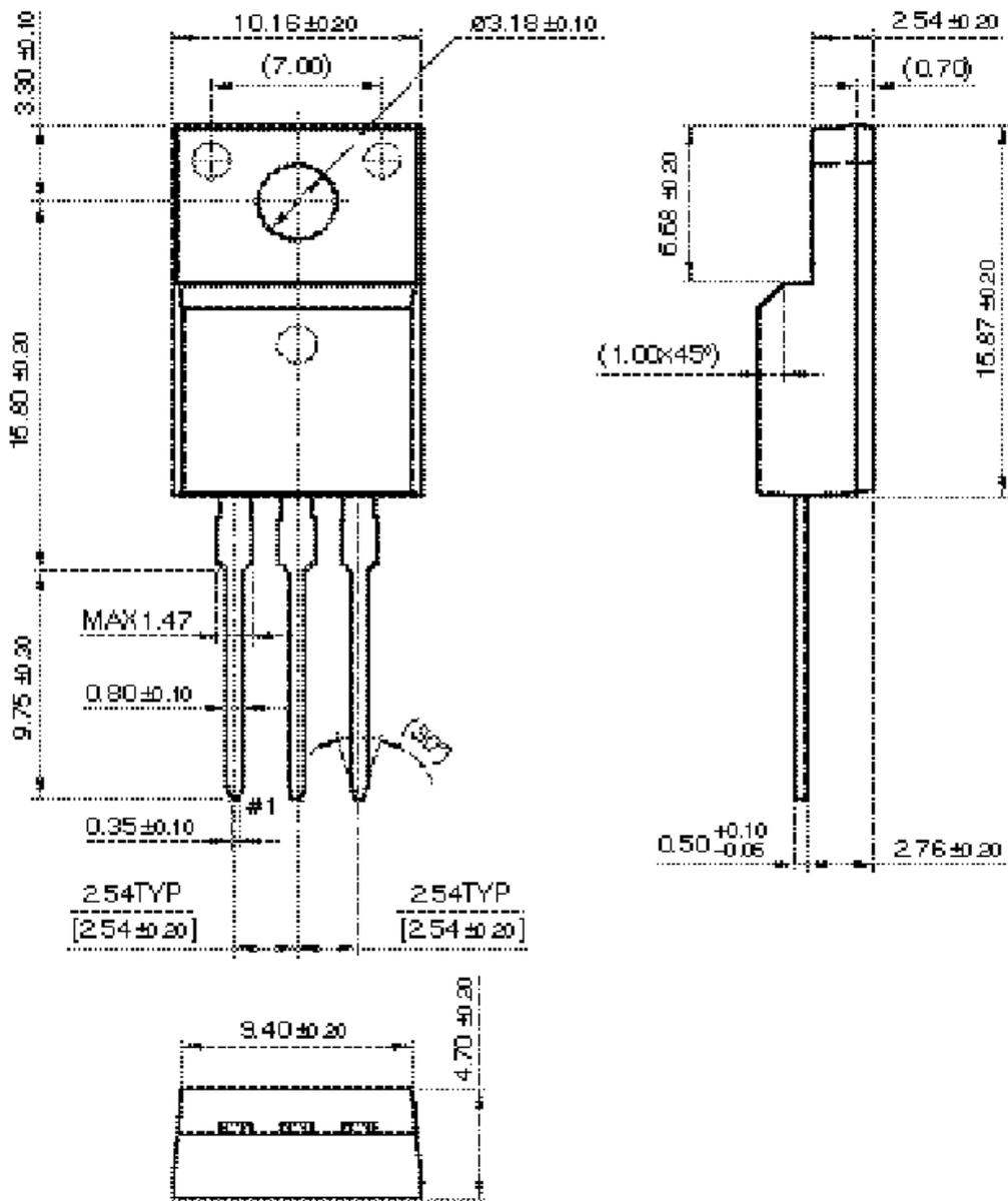
\* Front/Back Side Isolation Voltage : AC 2500V
