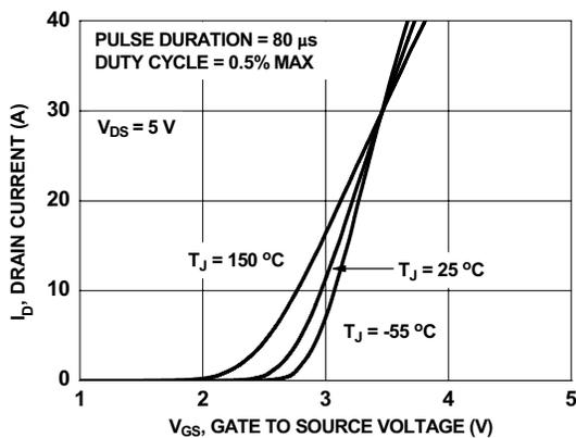
**Figure 5. Transfer Characteristics**
