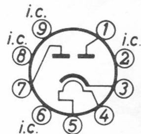
These two tubes are full-wave rectifiers. The EZ 81 has a noval base and a 6.3 volt, 1 amp heater. It can supply output currents of up to 150 millamps, and is therefore suitable for the AMPEREX 5-tube 10-watt amplifier circuit when the circuit is arranged for normal or low loading (plate to plate load 8000  $\Omega$  or 6000  $\Omega$ ), with or without a radio feeder unit.
