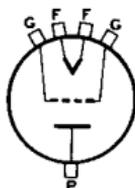
Grid terminals are spaced diametrically wider than filament terminals.
