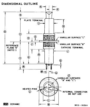
Reference plane "A" is defined as that plane against which annular surface "B" of the grid flange abuts.
