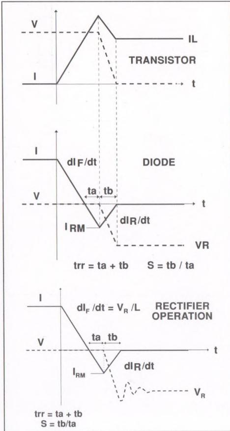
Fig. 8: TURN-ON CHARACTERISTICS
