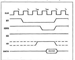
Figure 14 : Interrupt Acknowledge Timing.
