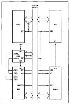
vicing an interrupt from any Z80 CTC channel. IEO blocks lower priority devices from interrupting while a higher priority interrupting device is being serviced.
