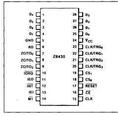
Figure 1 : Dual in Line Pin Configuration.
