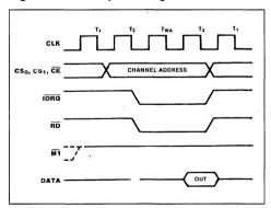
Low. M1 must be High to distinguish a write cycle from an interrupt acknowledge. A 2-bit binary code at inputs CS<sub>1</sub> and CS<sub>0</sub> selects the channel to be addressed, and the word being written is placed on the Z80 data bus. The data word is latched into the appropriate register with the rising edge of clock cycle  $T_3$ .
