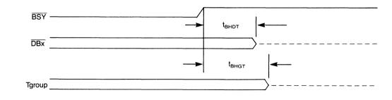
NOTE: Tgroup = signals driven by a Target =  $\overline{I/O}$ ,  $\overline{C/D}$ ,  $\overline{MSG}$ ,  $\overline{REQ}$
