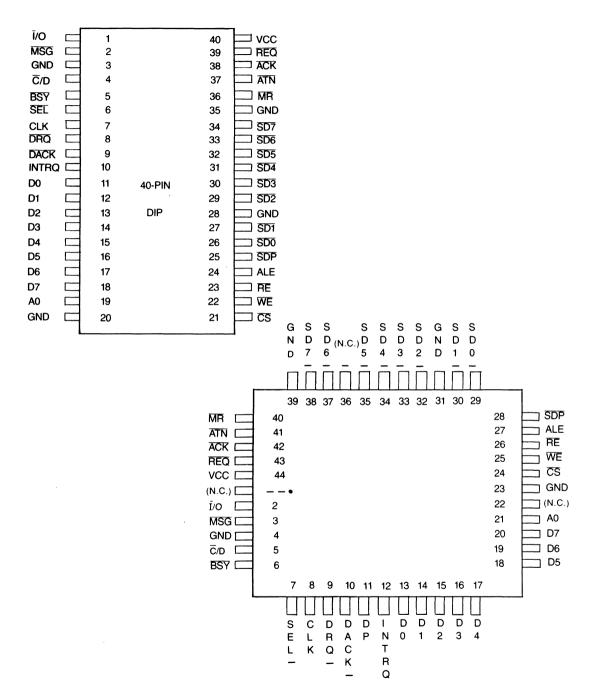
NOTE: Pin labeled N.C. should be left not connected.
