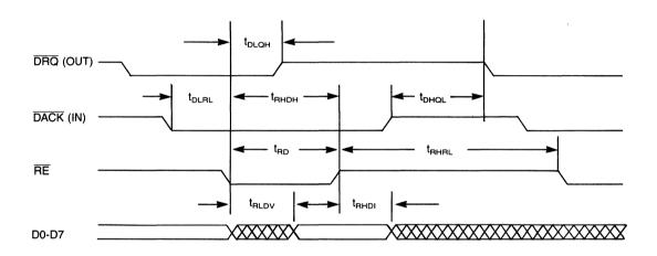
NOTE: External load on  $\overline{\text{DRQ}}$  & DACK is assumed to be 1KΩ.
