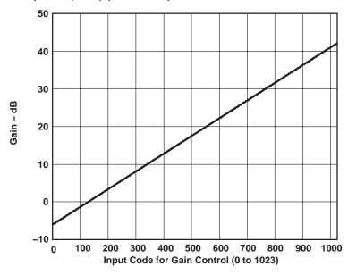
Figure 2. Characteristics of PGA Gain
