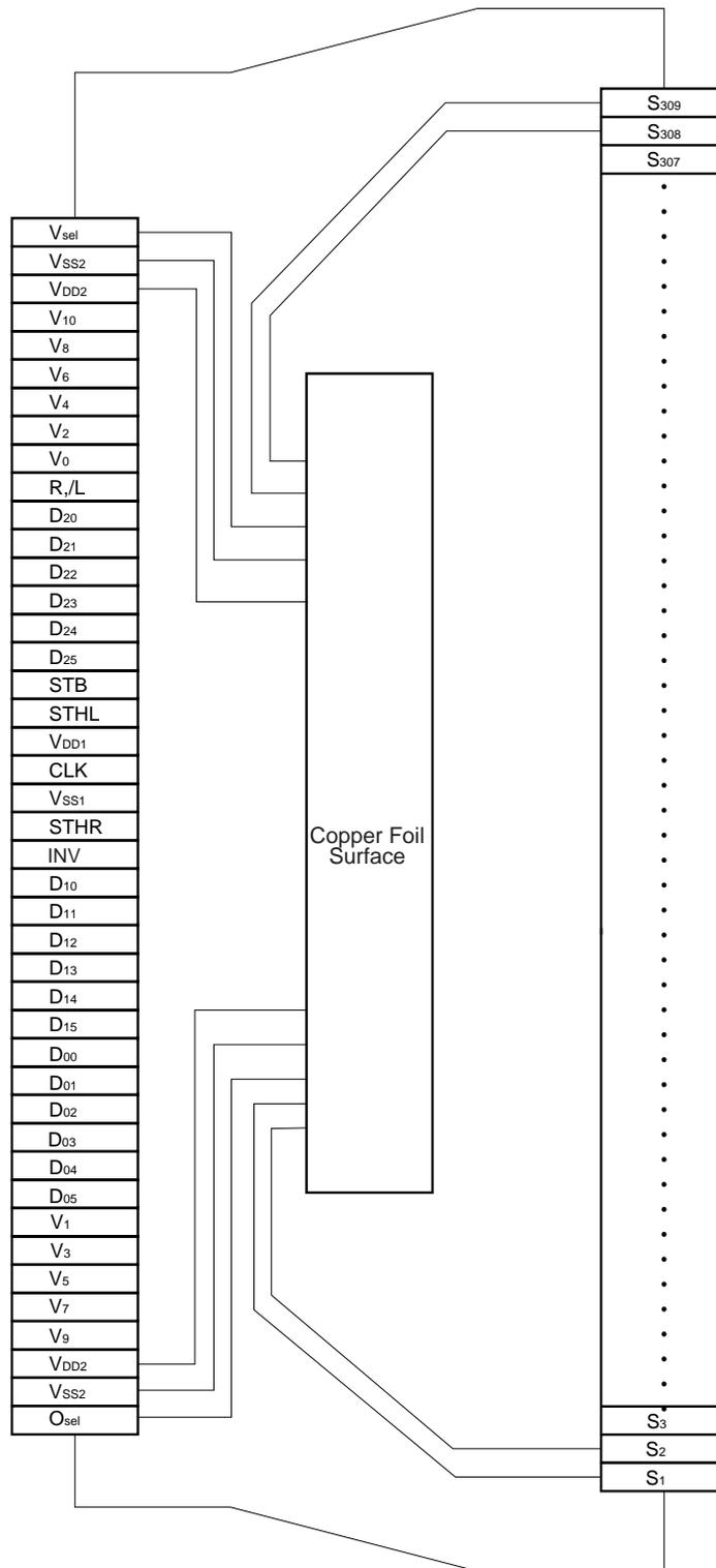
**Remark** O<sub>sel</sub> and V<sub>sel</sub> pins are internally pulled up.
