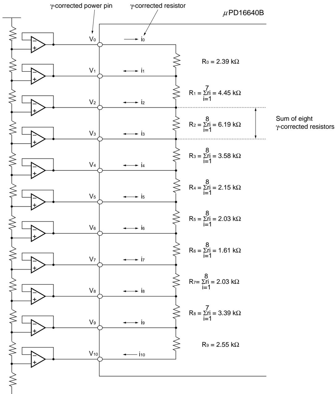
5. RELATIONSHIP BETWEEN OUTPUT CIRCUIT AND D/A CONVERTER
