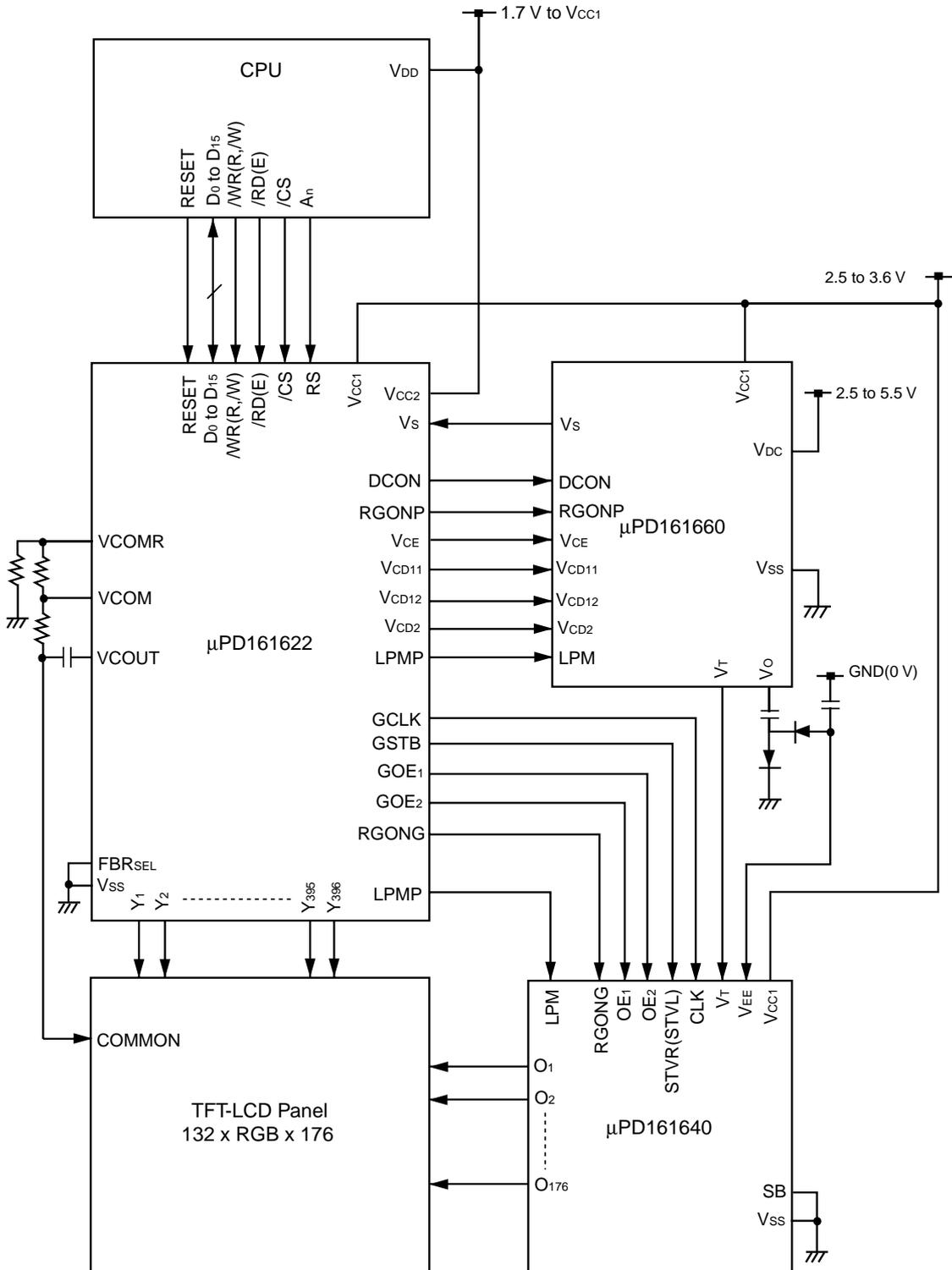
10. EXAMPLE of  $\mu$  PD161622 and CPU CONNECTION
