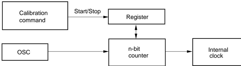
The calibration function involves counting the number of oscillation clocks generated between the start and stop signals and storing that number in a register. The number of oscillation clocks is then continually compared with this register value in subsequent operations, and the time of the clock number stored in the register is set as 1 line selection time, and used as the internal reference clock.
