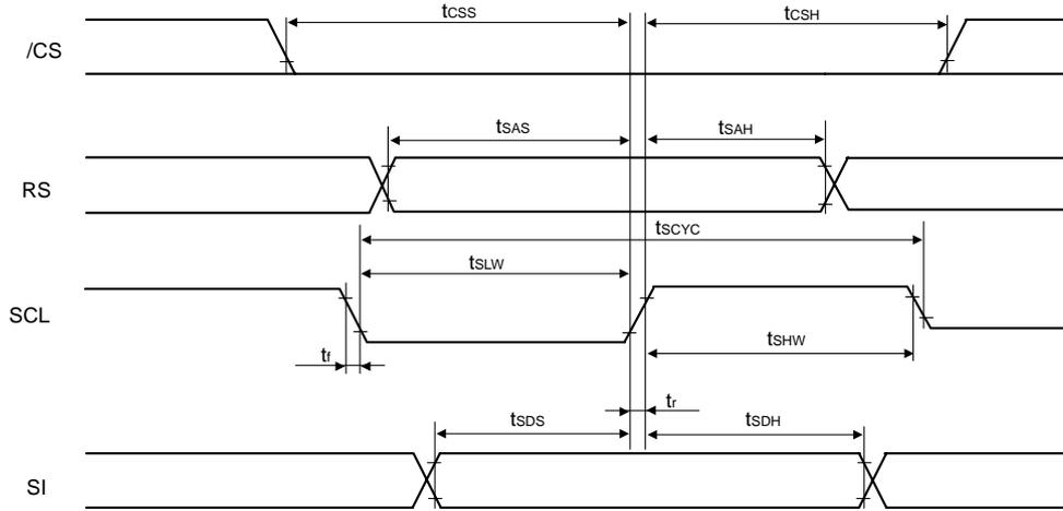
V<sub>CC1</sub> = 2.5 to 3.6 V, V<sub>CC2</sub> = 1.7 to 2.5 V, V<sub>CC1</sub> ≥ V<sub>CC2</sub>
