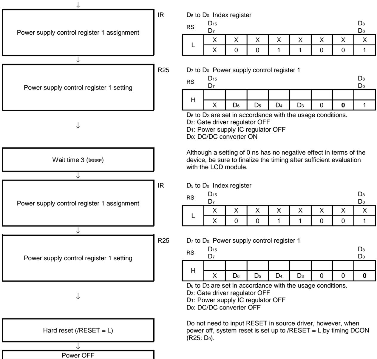
**Caution** This sequence is shown only for the purpose of illustrating the sequence up to when the power is turned off, and is not meant for use in mass-production design. Note also that this sequence differs depending on the configuration of the chipset and TFT-LCD module.
