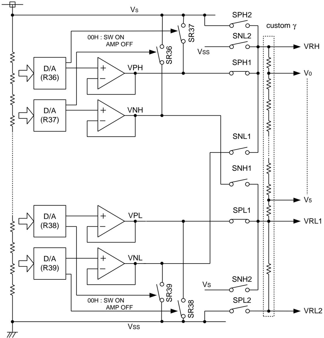
Figure 5–23. Relationship of TFT Drive Voltage (normally white)
