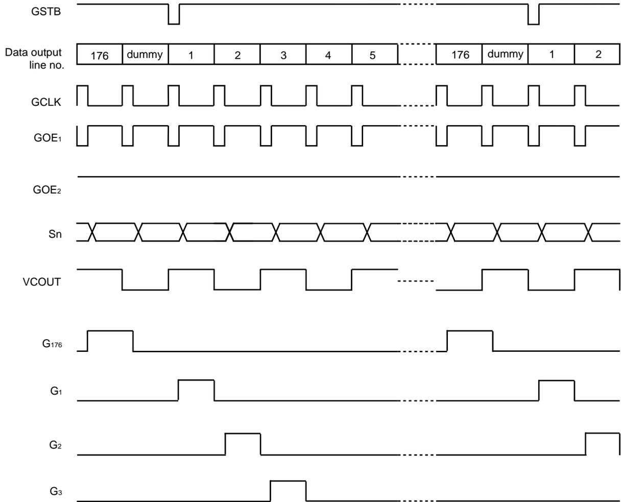
Figure 5-17. Normal Operation → Stand-by Input (during line inversion)
