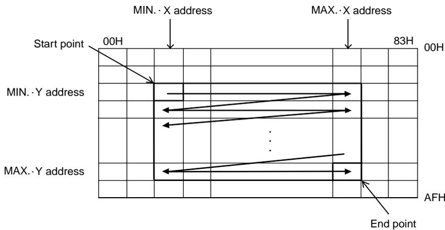
**Cautions 1. When using the window access mode, the relationship between the start point and end point shown in the table below must be established.**
