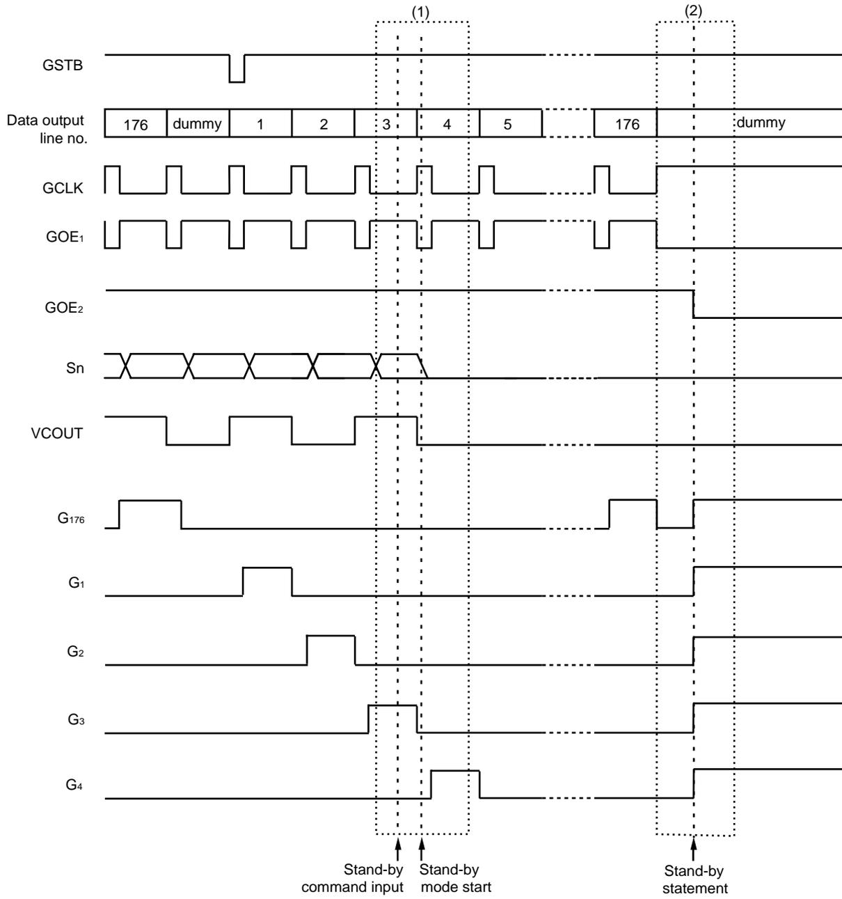
Figure 5-18. Normal Operation → Stand-by Input (during line inversion) (1) Reference
