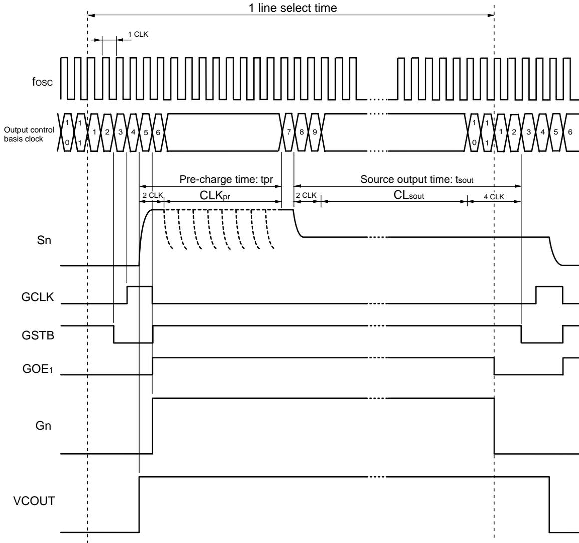
The display timing generator generates the timing signals for the internal timing of the source driver and for the gate driver. The output timings for normal operation, for normal operation → stand-by mode, and for stand-by mode → normal operation, are shown below.
