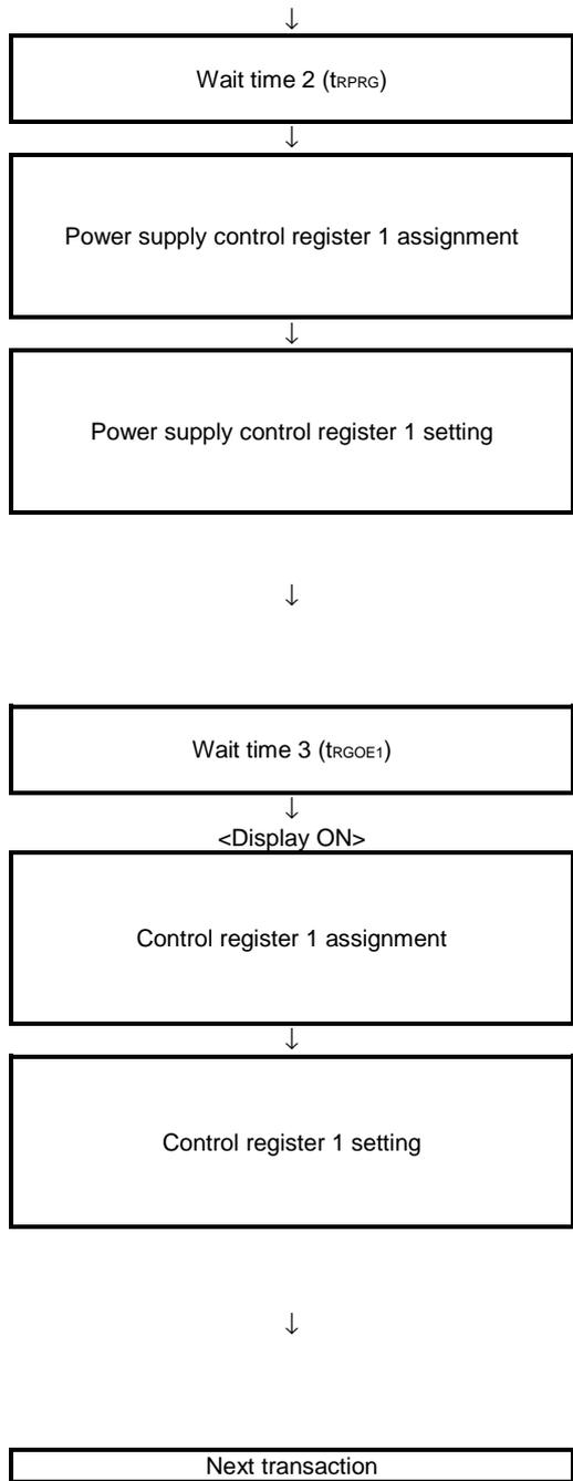
trPRG is the output stable period of the DC/DC converter. Although a setting of about 20 mS is the target, be sure to finalize the timing after sufficient evaluation with the LCD module.
