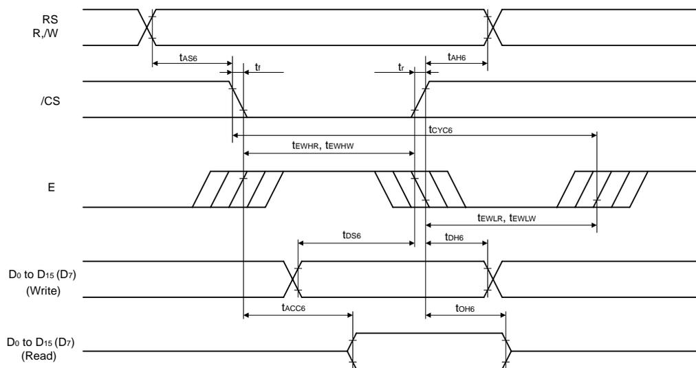
When V<sub>CC1</sub> = 2.5 to 3.6 V, V<sub>CC2</sub> = 2.5 to 3.6 V, V<sub>CC1</sub> ≥ V<sub>CC2</sub> (normal mode, R114 and R115 = 03H)
