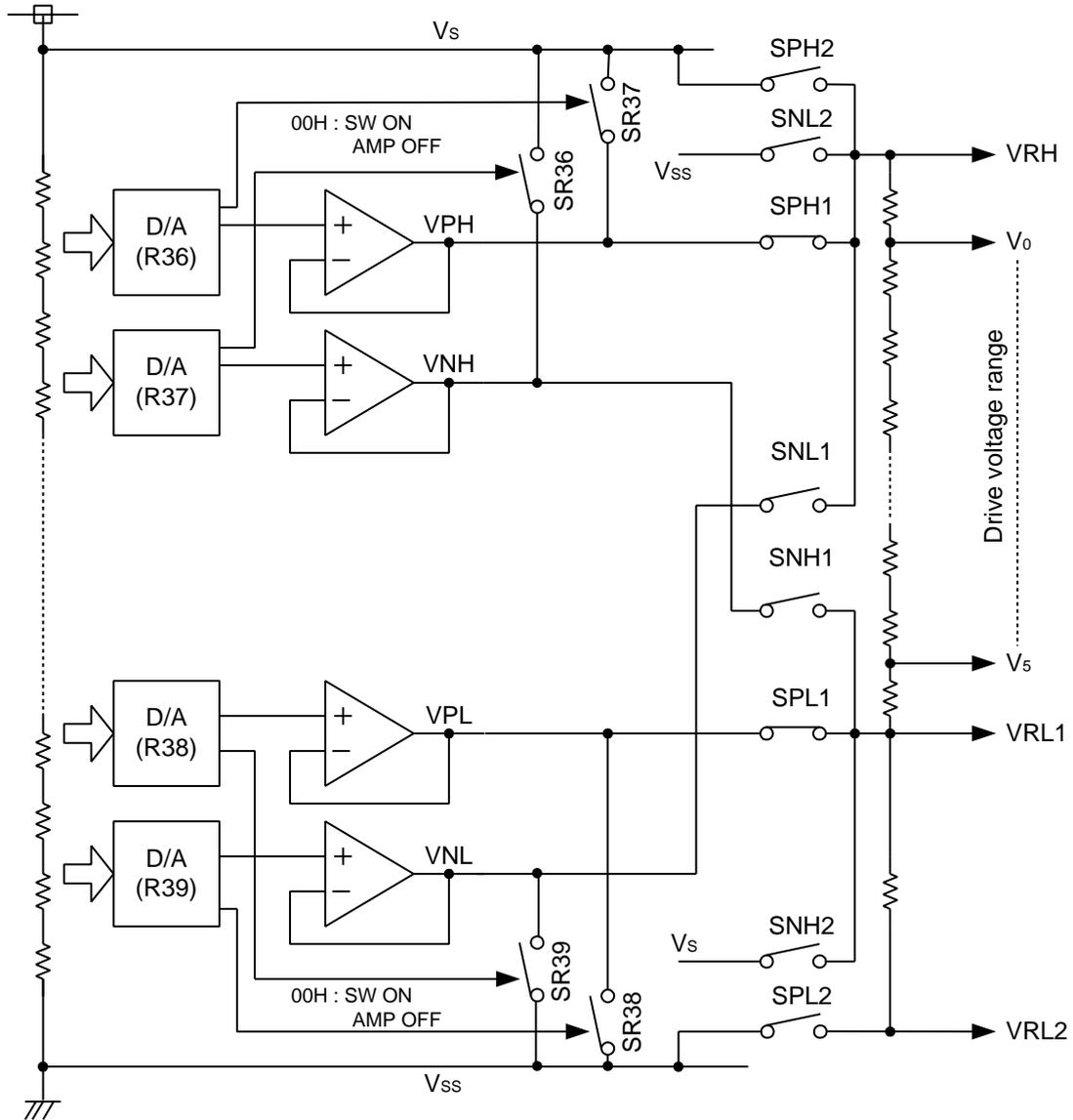
Table 5-14. γ-Curve Correction Circuit (γ-correction resistance)
