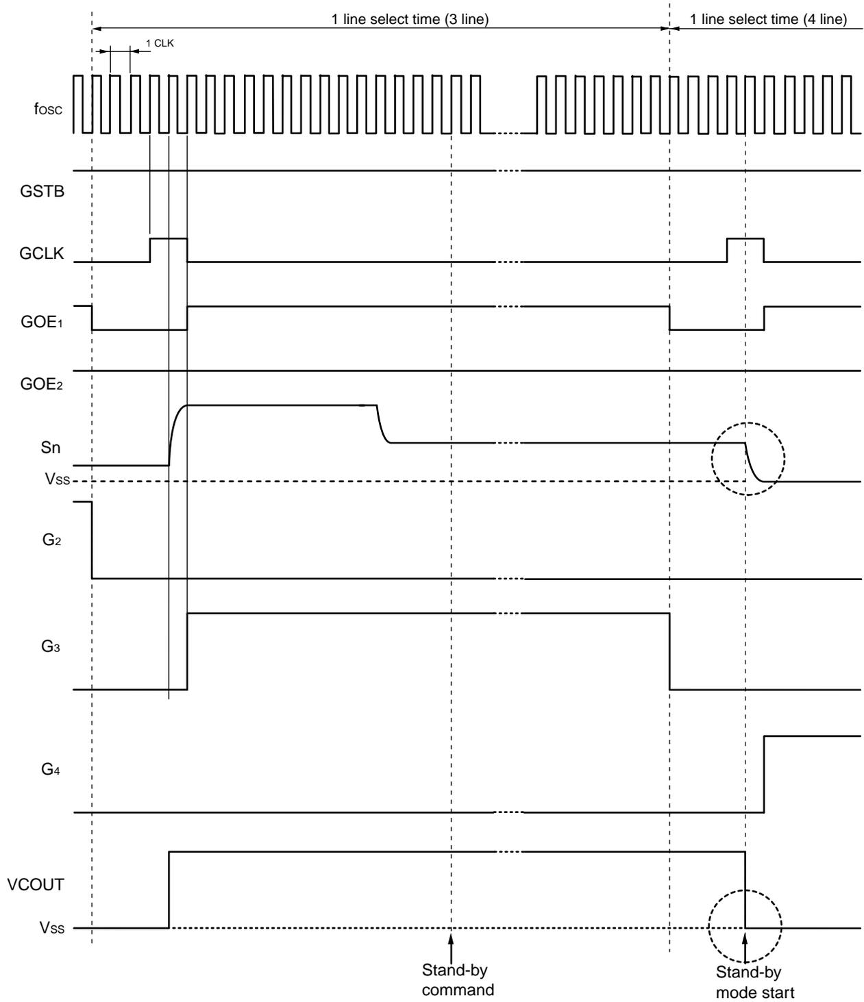
Figure 5-19. Normal Operation → Stand-by Input (during line inversion) (2) Reference
