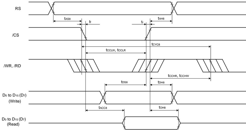
**When V<sub>CC1</sub> = 2.5 to 3.6 V, V<sub>CC2</sub> = 2.5 to 3.6 V, V<sub>CC1</sub> ≥ V<sub>CC2</sub> (normal write mode, R114 and R115 = 03H)**
