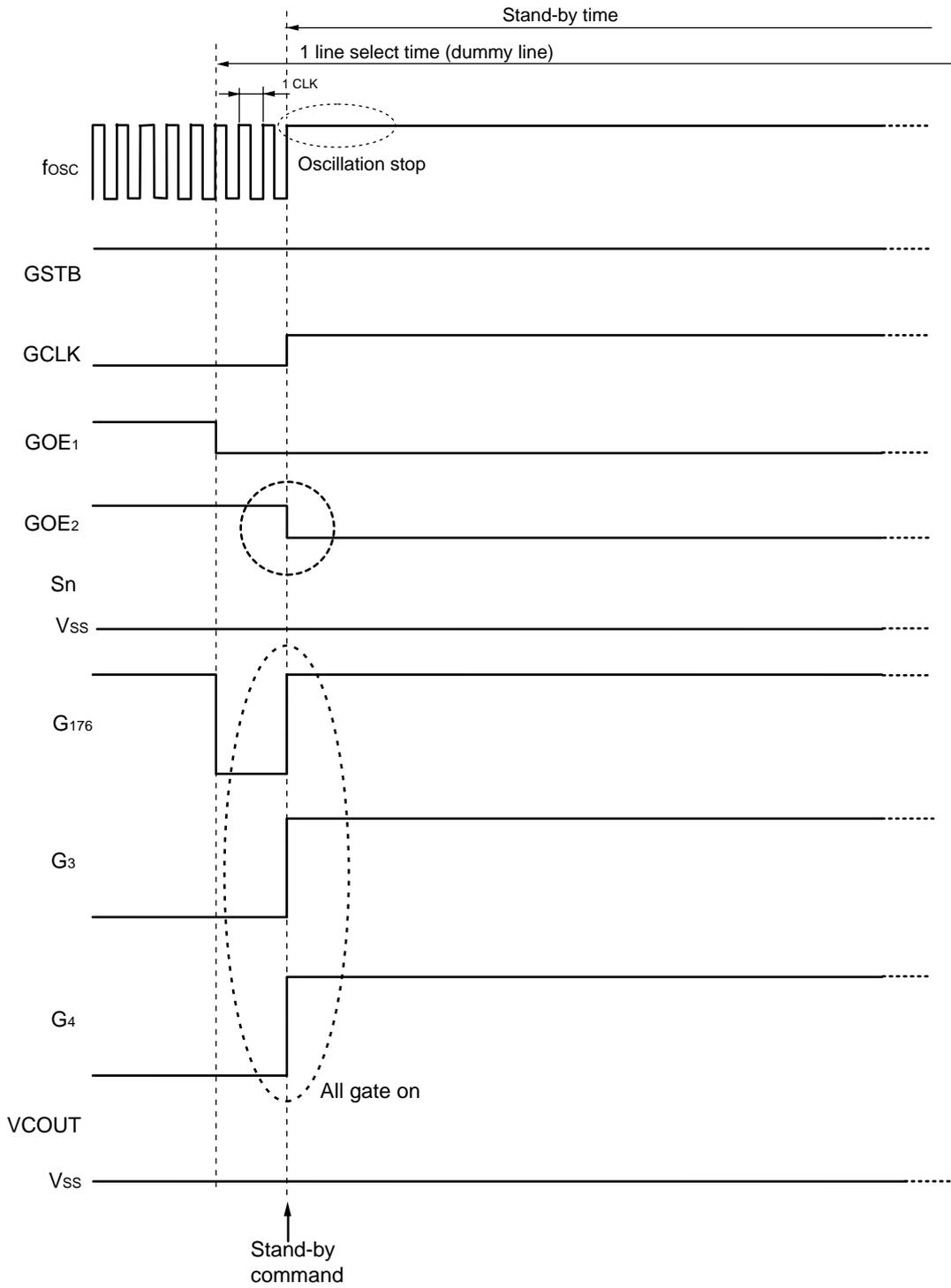
Figure 5-20. Stand-by → Return to Normal Operation (during line inversion)
