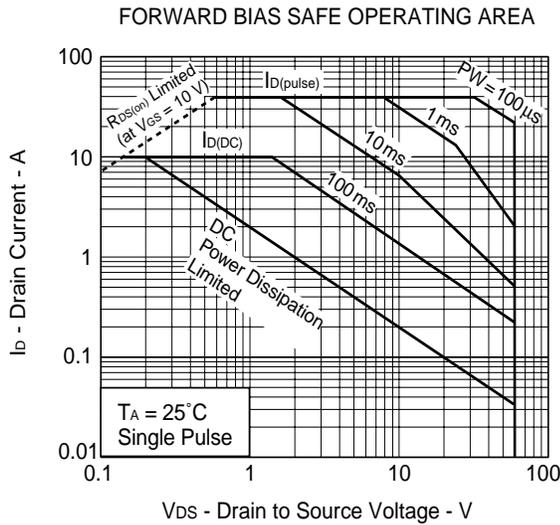
Remark Mounted on ceramic substrate of 1200 mm<sup>2</sup> × 2.2 mm
