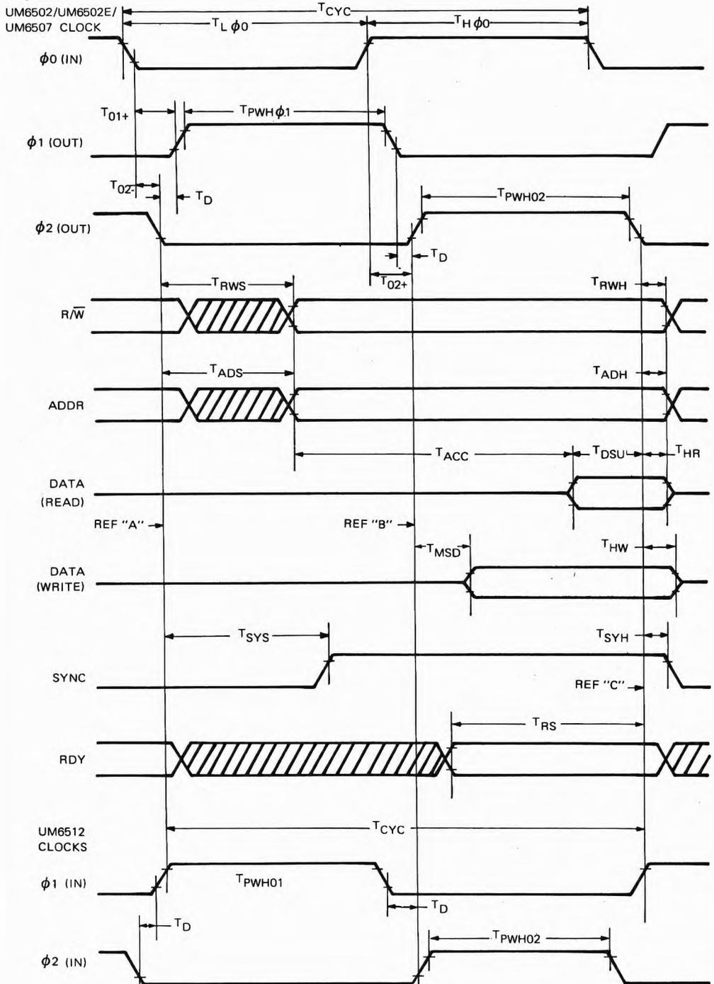
**Dynamic Operating Characteristics** ( $V_{CC} = 5.0 \pm 5\%$ ,  $T_A = 0^\circ$  to  $70^\circ\text{C}$ )
