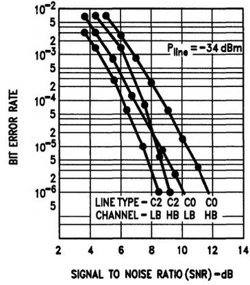
**FIGURE 2. Bit Error Rate vs Signal-to-Noise Ratio**
