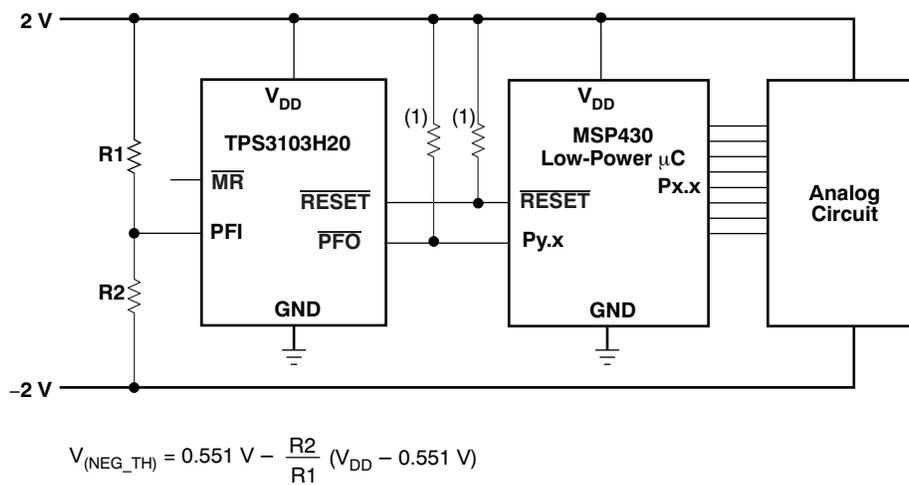
(1) Resistor may be integrated in  $\mu\text{C}$ .
