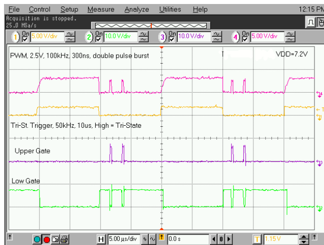
Figure 21. 2.5-V Amplitude PWM Pulse
