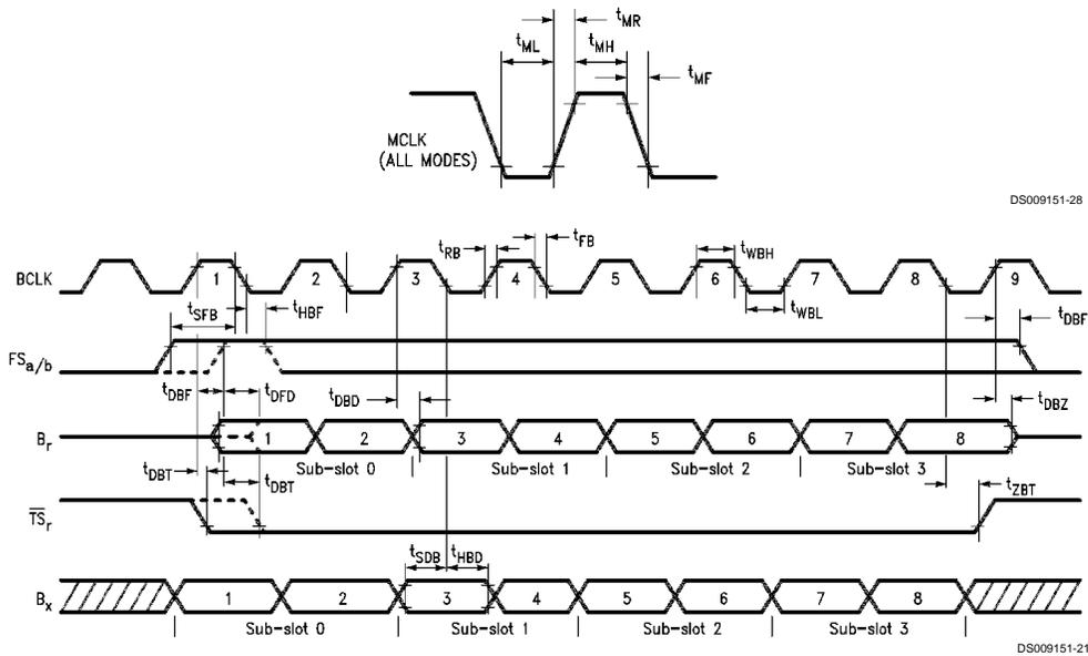
FIGURE 18. Non-Delayed Data Timing Mode (Formats 1 and 3)
