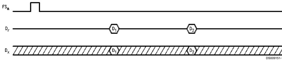
FIGURE 11. D-Port Interface Timing Using BCLK Format 2
