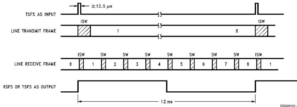
FIGURE 2. Superframe Sync Pin Timing
