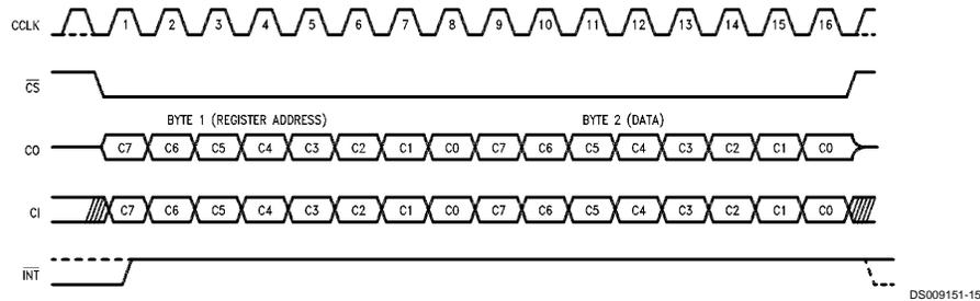
FIGURE 13. Microwire Control Port Timing: MW = 1
