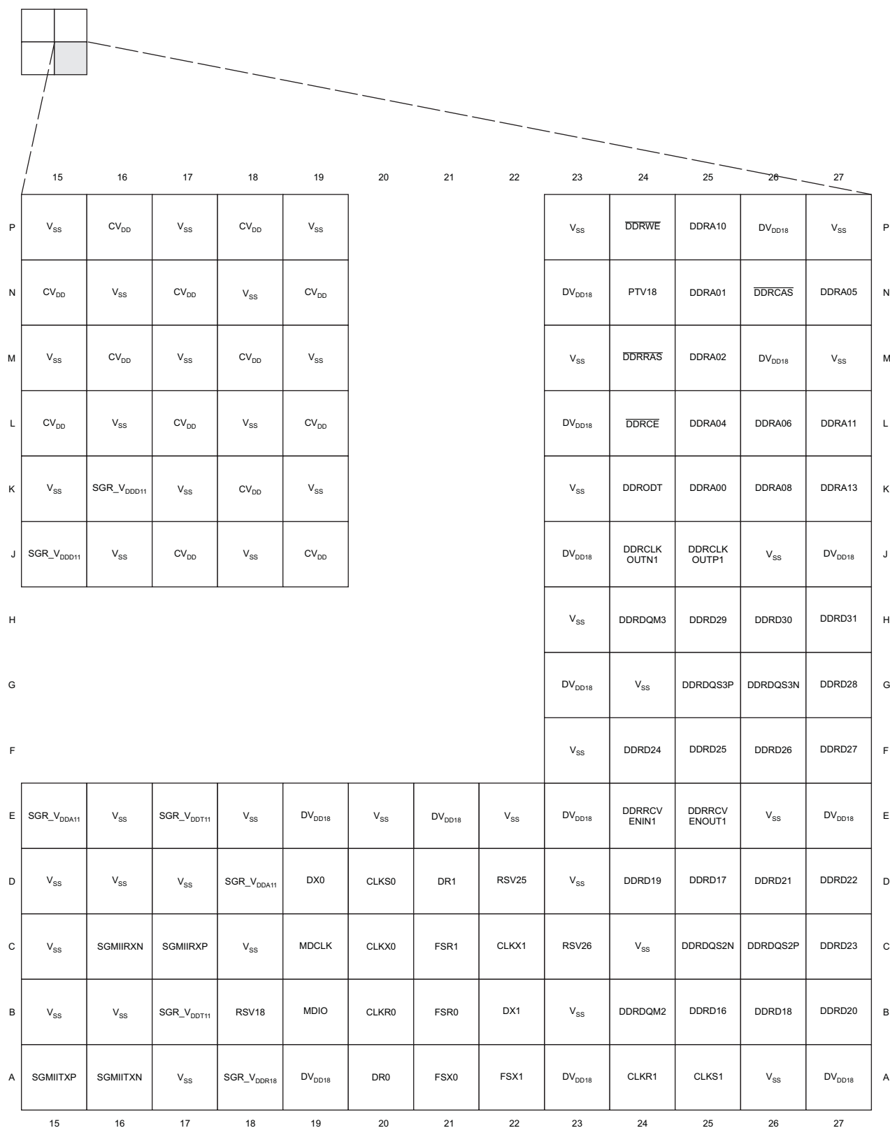
Figure 2-4. TCI6487/8 Pin Map (Bottom View) [Quadrant C]
