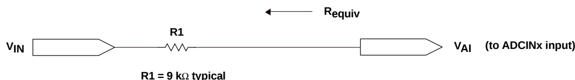
Figure 48. Typical ADC Input Pin Circuit
