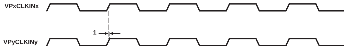
Figure 5-57. Video Port Dual-Display Sync Timing
