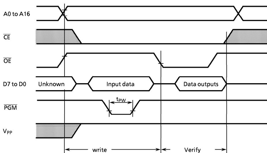
**Note1:** When  $V_{CC}$  power supply is turned on or after,  $V_{PP}$  must be increased.
