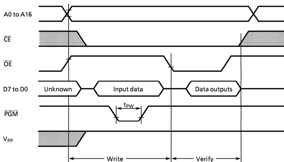
**Note 1:** The power supply of  $V_{PP}$  (12.75 V) must be set power-on at the same time or the later time for a power supply of  $V_{CC}$  and must be clear power-on at the same time or early time for a power supply of  $V_{CC}$ .
