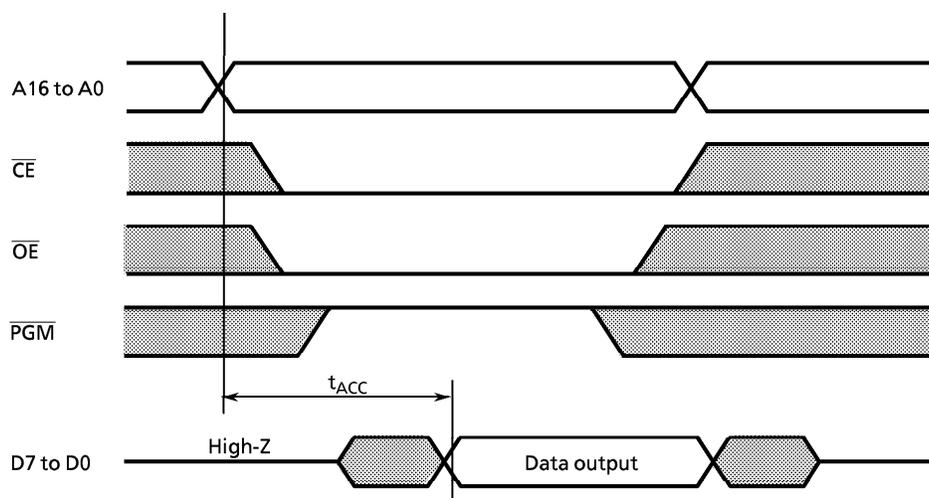
(2) Program operation (High-speed) ( $T_{opr} = 25 \pm 5^{\circ}\text{C}$ )
