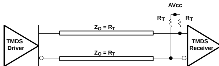
Figure 1. Termination for TMD5 Output Driver
