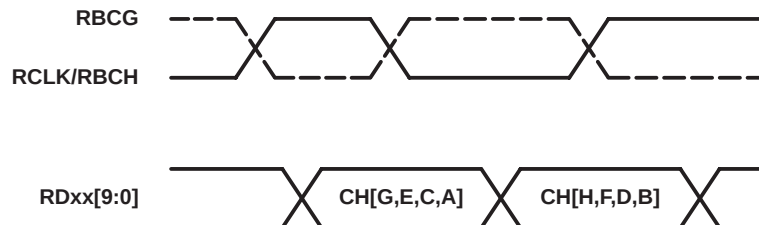
Figure 6. Multiplexed Channel Receive Timing
