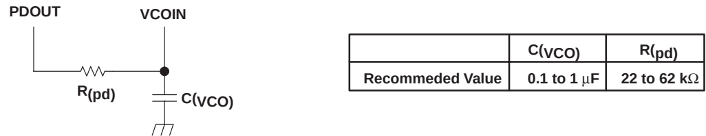
Figure 8. Resistor and Capacitor Connection
