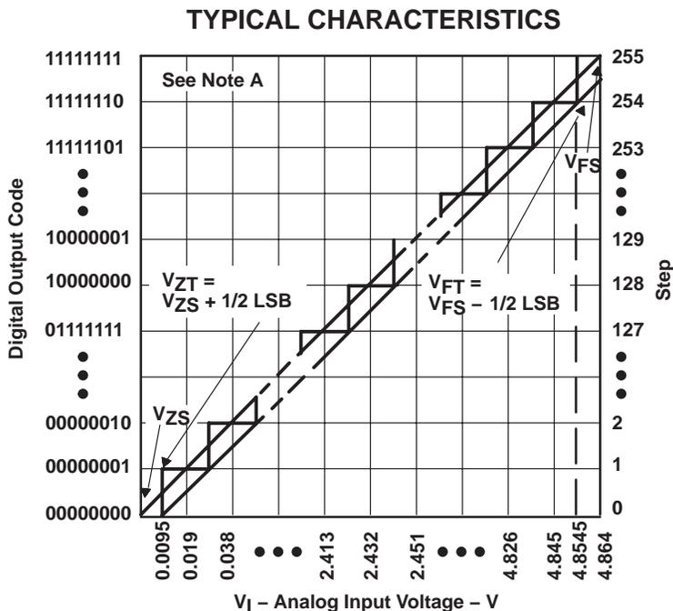
NOTE A: This curve is based on the assumption that  $V_{refB}$  and  $V_{refT}$  have been adjusted so that the voltage at the transition from digital 0 to 1 ( $V_{ZT}$ ) is 0 and the transition to full scale ( $V_{FT}$ ) is 4.8545 V. 1 LSB = 19 mV.
