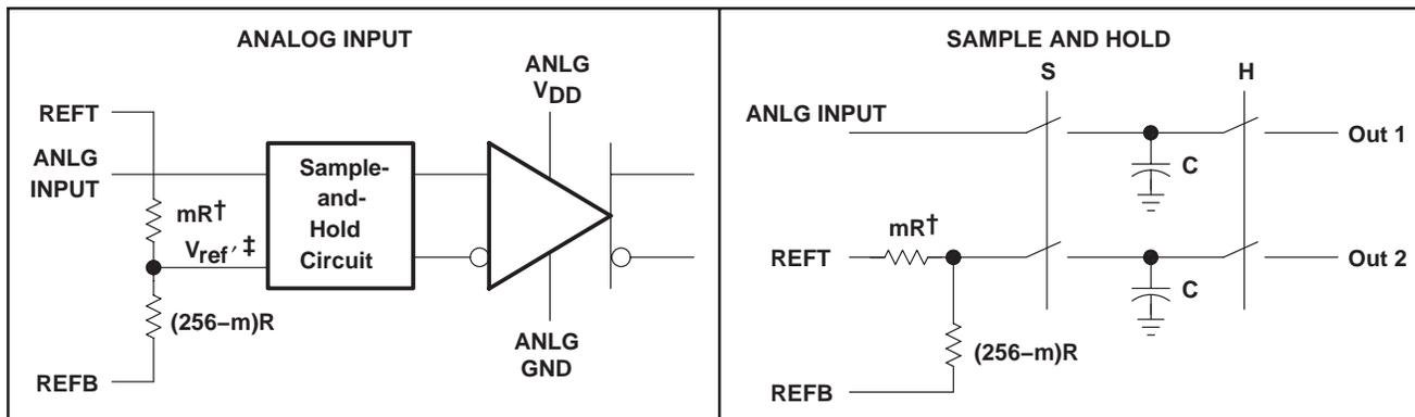
† m = comparator position along the resistor string
