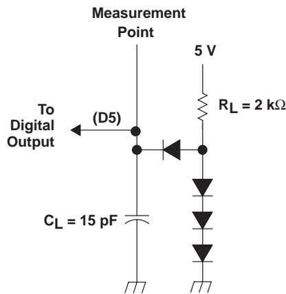
Figure 10. Load Circuit
