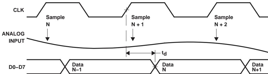
Following the operating sequence above, the rising edge of the clock samples the analog input (sample N) at time  $t_N$  and latches sample N-1 at the output. Sample N is encoded to eight digital lines on the next falling edge of the clock and then the following high clock level latches these eight bits to the outputs (with a delay  $t_d$ ) and acquires sample N + 1. Conversion is completed in one clock cycle and continues the sequence for the next cycle.
