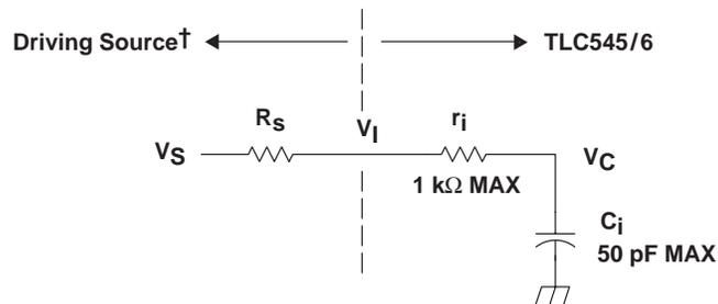
$V_I$  = Input Voltage at INPUT A0–A18
