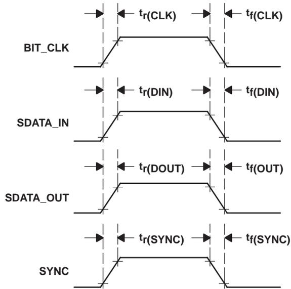
Figure 4-4. Signal Rise and Fall Timing
