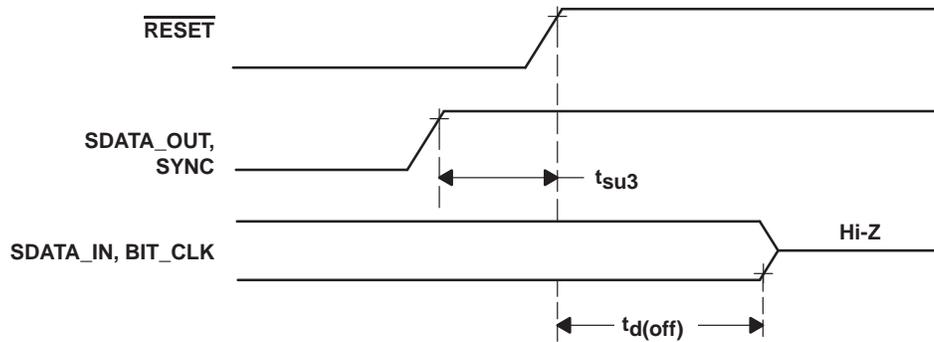
Figure 4-7. ATE Test Mode Timing
