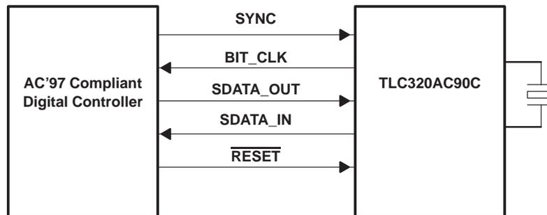
Figure 5–2. Connection to an AC'97 Digital Controller
