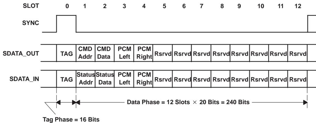
Figure 2–1. AC-Link Bidirectional Audio Frame (As Implemented)
