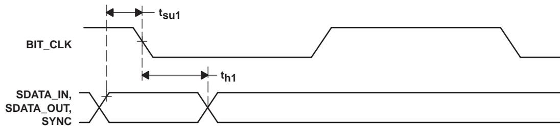
Figure 4-3. Data Setup and Hold Timing
