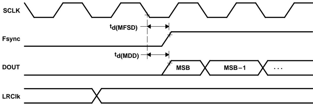
Figure 4-1. SCLK to Fsync and DOUT – Master Mode 3
