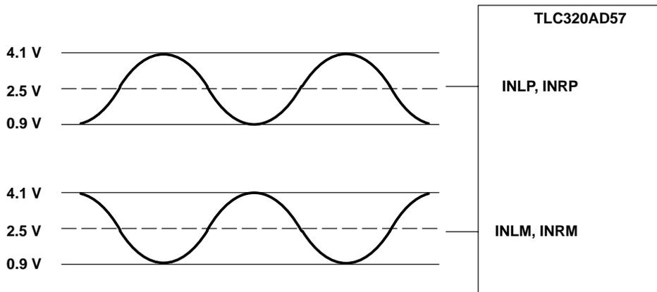
Figure 2–2. Differential Analog Input Configuration
