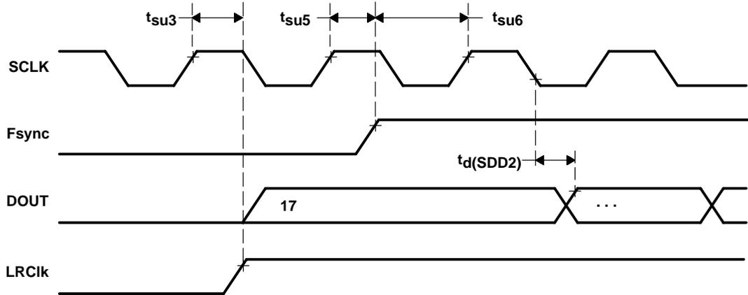
Figure 4-6. SCLK to Fsync, LRCIk, and DOUT – Slave Mode 2, Fsync Controlled
