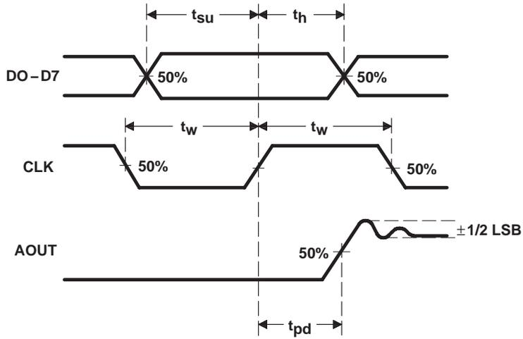
Figure 1. Voltage Waveforms
