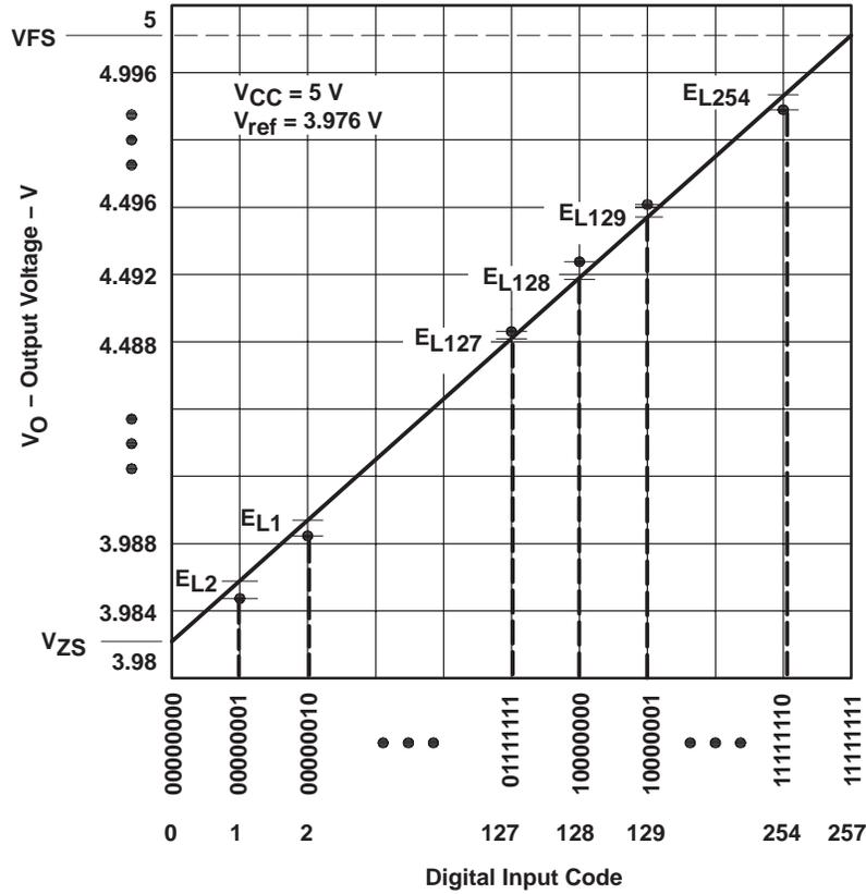
Figure 3. End-Point Linearity Error
