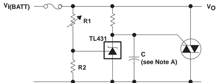
NOTE A: Refer to the stability boundary conditions in Figure 16 to determine allowable values for C.
