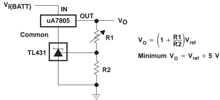
Figure 20. Output Control of a 3-Terminal Fixed Regulator
