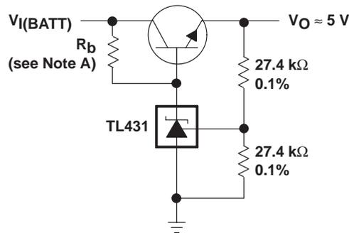
NOTE A:  $R_b$  should provide cathode current  $\geq 1$ -mA to the TL431.
