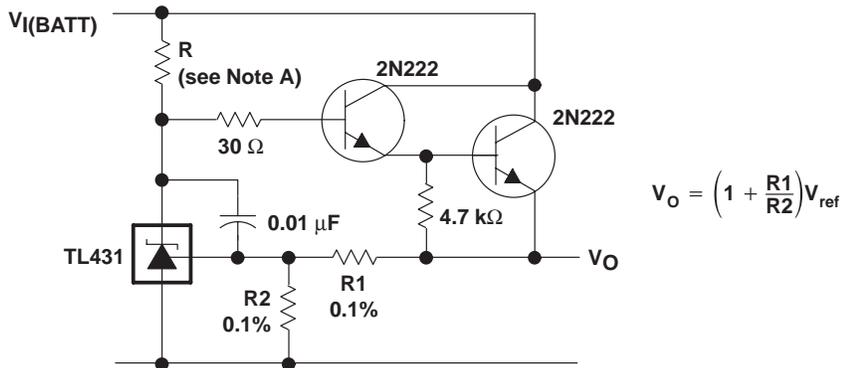
NOTE A: R should provide cathode current  $\geq 1$  mA to the TL431 at minimum  $V_{I(BATT)}$ .
