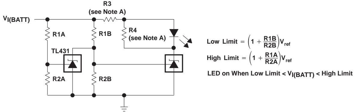
NOTE A: R3 and R4 are selected to provide the desired LED intensity and cathode current  $\geq 1$  mA to the TL431 at the available  $V_{I(BATT)}$ .
