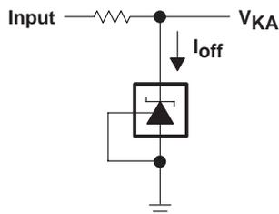
Figure 4. Test Circuit for  $I_{\text{off}}$
