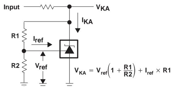
Figure 3. Test Circuit for  $V_{\text{KA}} > V_{\text{ref}}$
