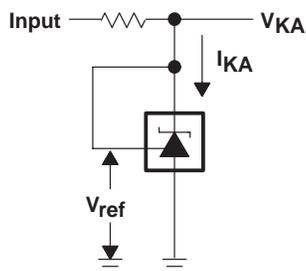
Figure 2. Test Circuit for  $V_{\text{KA}} = V_{\text{ref}}$
