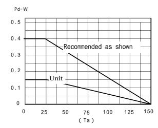
Approximate power dissipation is 400 mW at 25 Derating value is 3.2 mW / over 25 ( ja = 312 / W )
