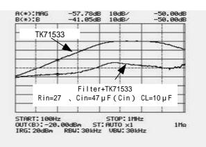
$R{=}27~$   $C{=}47\,\mu\,F$  (electrolysis) There are no characteristic changes in (Iout=20, 30, and 40mA)
