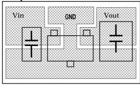
PCB: Glass epoxy 30 \* 30mm t=0.8mm
