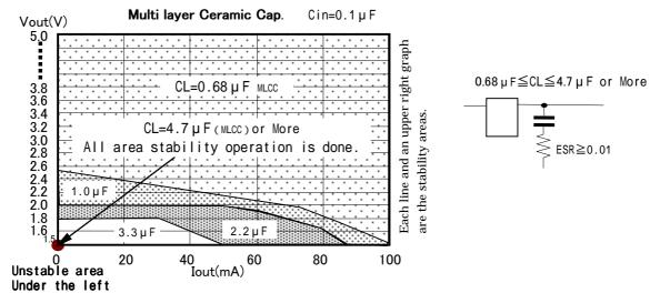
Range which can be used :Vo≥2.8V Io=1mA~Max, Multi layer Ceramic Cap.≥0.68 µ F :Vo≥2.0V Io=1mA~Max, Multi layer Ceramic Cap.≥1.0 µ F :Vo≥1.5V Io=1mA~Max, Multi layer Ceramic Cap.≥4.7 µ F
