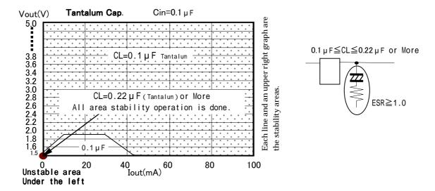
Range which can be used: Vo $\geq$ 1.9V Io=1mA $\sim$ Max, Tantalum Cap. $\geq$ 0.1  $\mu$ F or (Ceramic Cap. 0.22  $\mu$ F +2.2  $\Omega$ ) : Vo $\geq$ 1.5V Io=1mA $\sim$ Max, Tantalum Cap. $\geq$ 0.22  $\mu$ F or (Ceramic Cap. 0.22  $\mu$ F +2.2  $\Omega$ )
