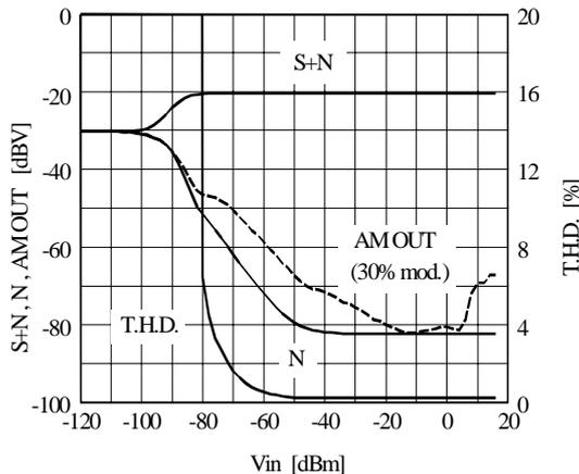
Detector output vs Mixer input level
