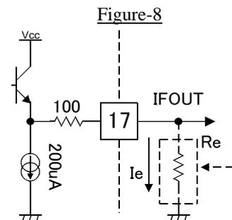
RSSI output is the current output. It is converted the voltage by an external resistor between Pin 18 and GND. The time constant of RSSI output is determined by the product of an external converting resistance and parallel capacitance. The time constant is longer, RSSI output is harder to be influence by the disturbance or the ingredient of amplitude modulation, but RSSI output response is slower. Determine the external resistance and capacitance with the purpose.
