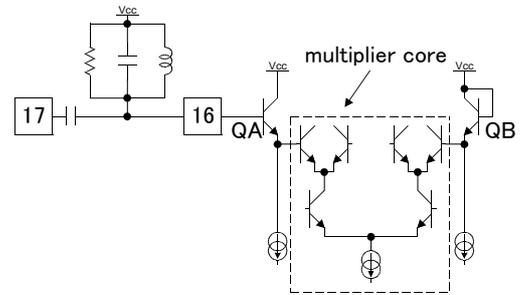
Figure-12 the examples of phase shifter
