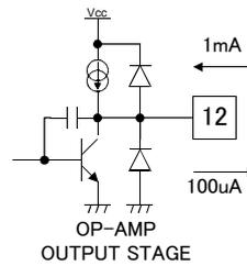
Figure-15 the internal equivalent circuit of comparator output stage. As comparator output is an open collector, it is suitable for the many interface level. This open collector output is connected with an electrostatic discharge protection diode at GND side only, but not connected with it at a power supply side in consideration of operating the voltage over the supply voltage of this IC.
