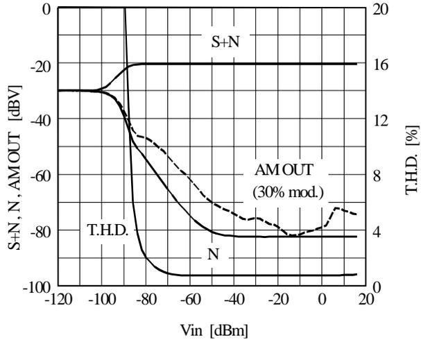
**RSSI Output Voltage vs Input Voltage**
