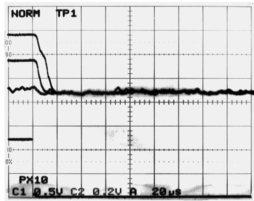
**RSSI OUTPUT VOLTAGE TRANSIENT RESPONSE - POWER SAVE ON/OFF**
