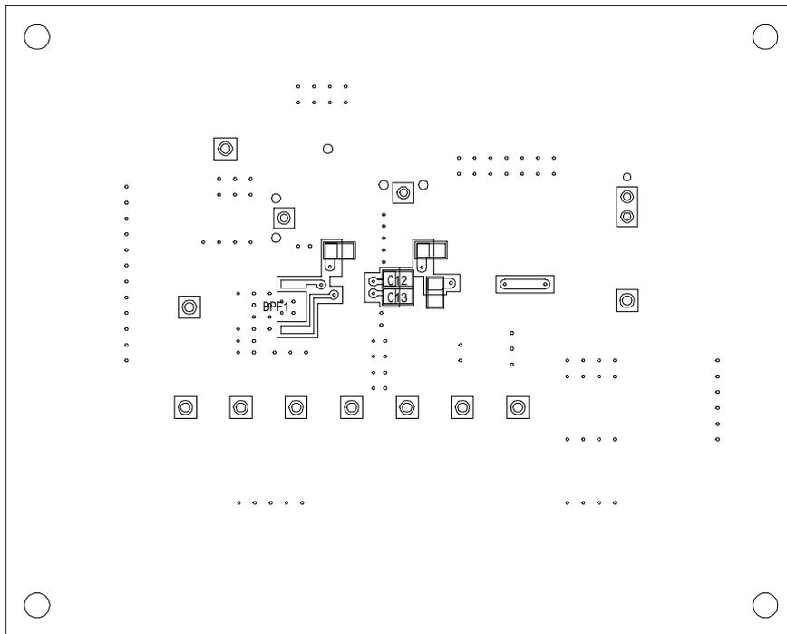
C2=C3=C4=C6=C8=C9=C10=C11=C12=C13=0.01uF, C1=4.7uF, C5=100pF, C7=1pF, R1=R6=51, R2=3k, R3=100, R4=2k, R5=18k, L1=L2=10uH, L3=836BH-0268 (TOKO), BPF=ESK107MA-AE-10(TOKO)
