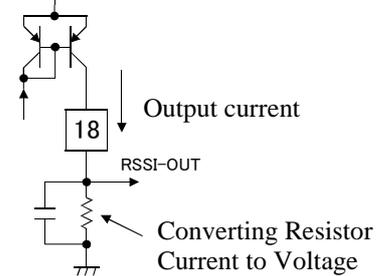
AM demodulation by using the RSSI output
