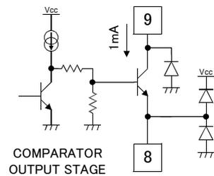
Please the reference terminal of comparator input is used the side of minus terminal (Pin 10) certainly. In case the reference terminal is used the side of plus terminal (Pin 11), it is feared that the comparator output oscillates.
