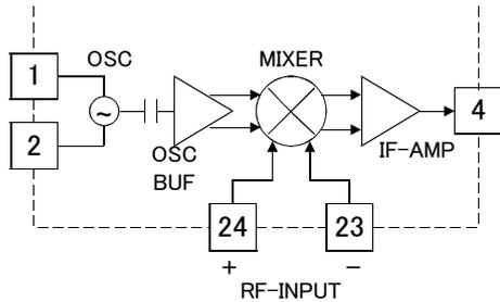
As RF input is the balance input, it is easy to match the SAW filter etc.
