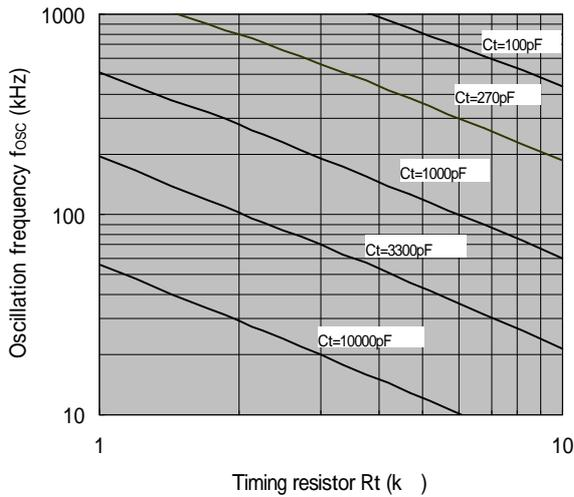
Fig.3: Oscillator frequency vs. Timing resistor
