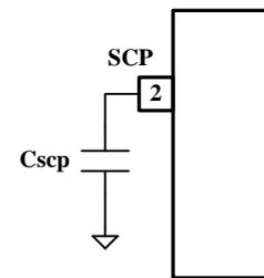
Fig 10. SCP pin connection
