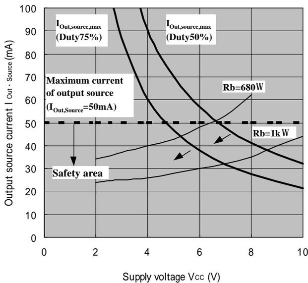
Fig 9. Output source current vs. supply voltage
