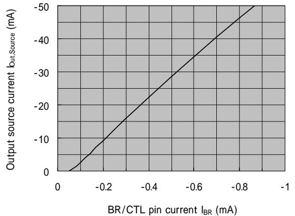
Fig 8. Output source current vs. BR/CTL pin current
