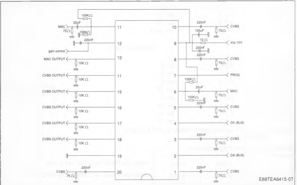
**Note :** When any input is not used, it must be bypassed to ground through a 220nF capacitor, so as to avoid degrading the crosstalk.
