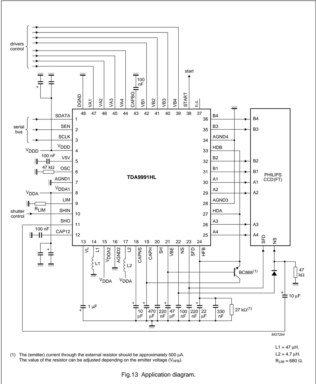
Vertical line driver and DC-DC converter for
