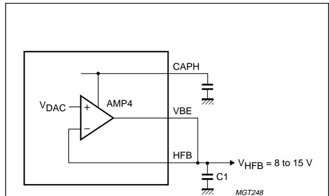
Fig.8 Principle of voltage regulator of drivers supply in mode 2.
