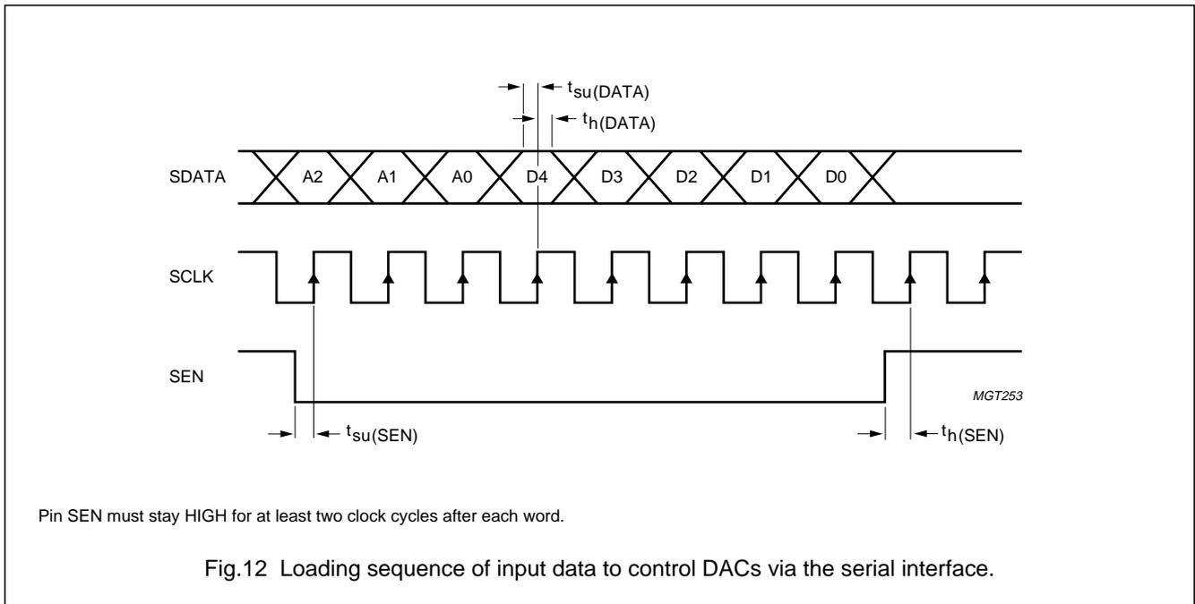
Pin SEN must stay HIGH for at least two clock cycles after each word.
