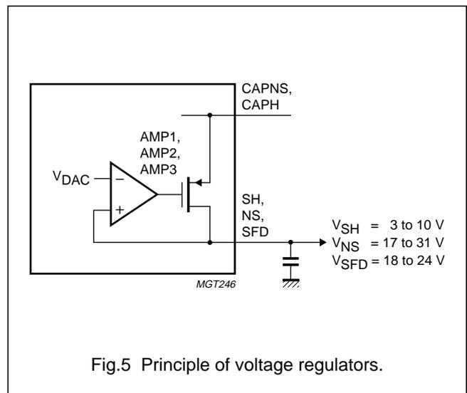
Fig.5 Principle of voltage regulators.
