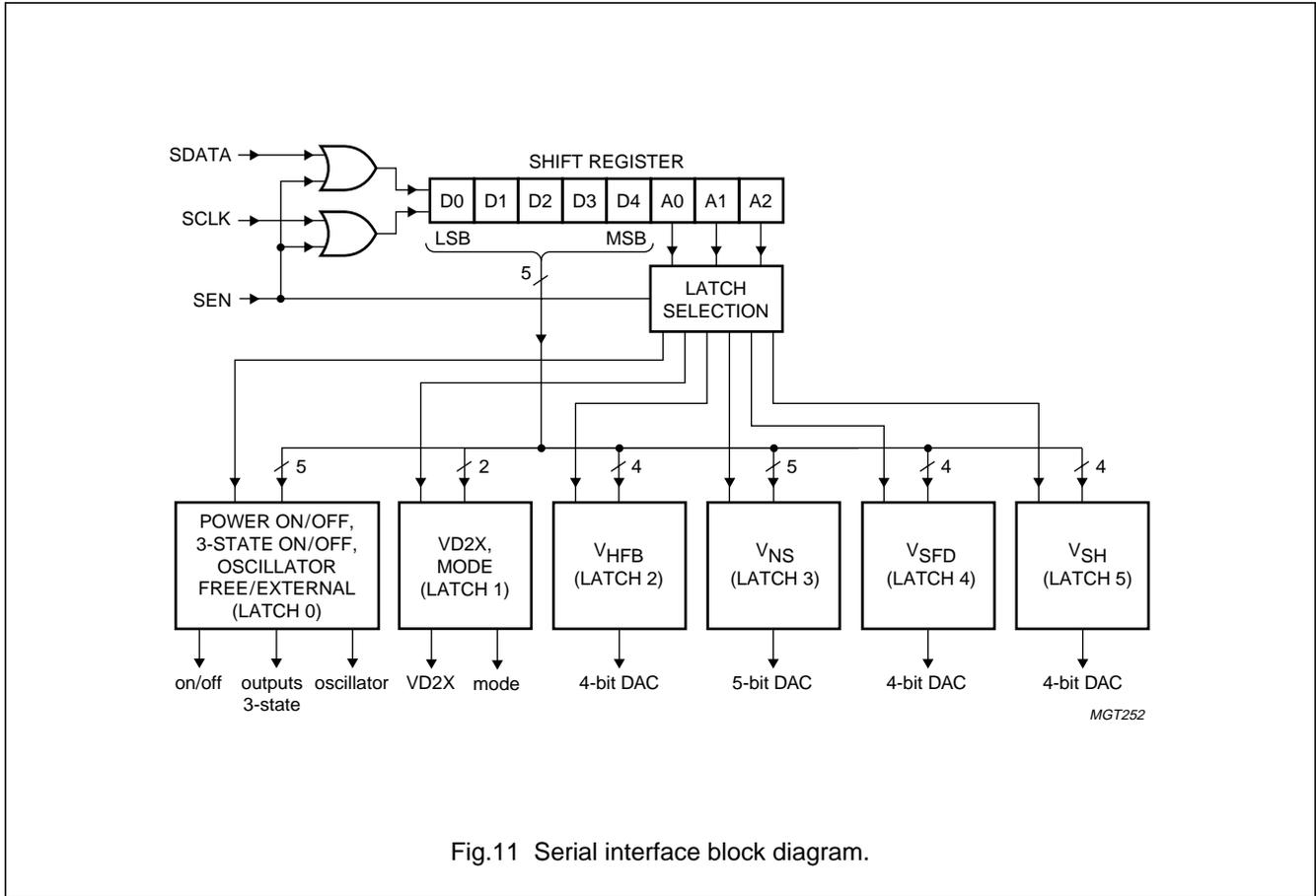
Fig.11 Serial interface block diagram.
