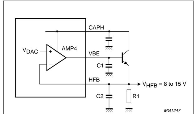
Fig.6 Principle of voltage regulator of drivers supply in mode 1.
