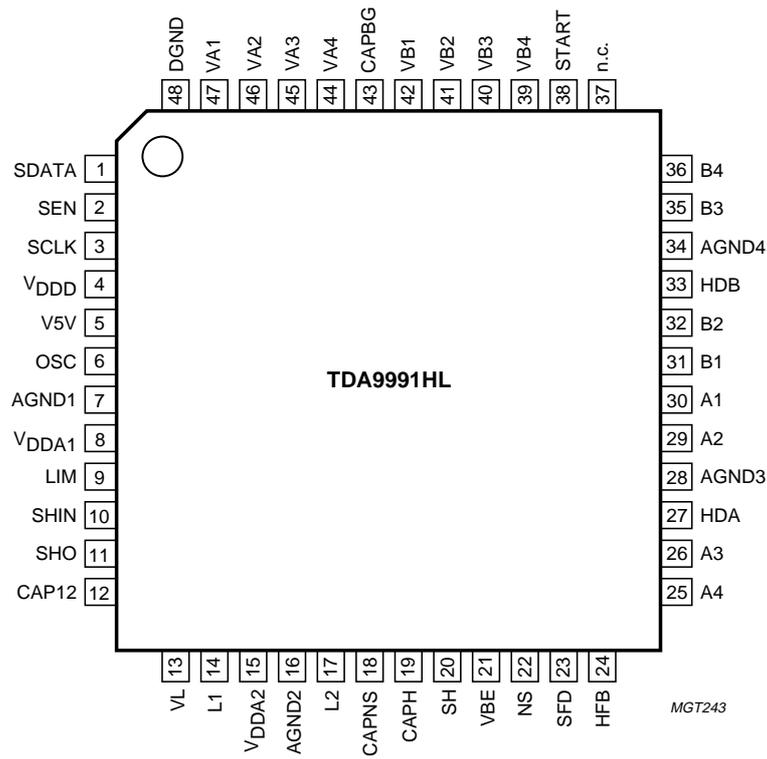
Fig.2 Pin configuration.
