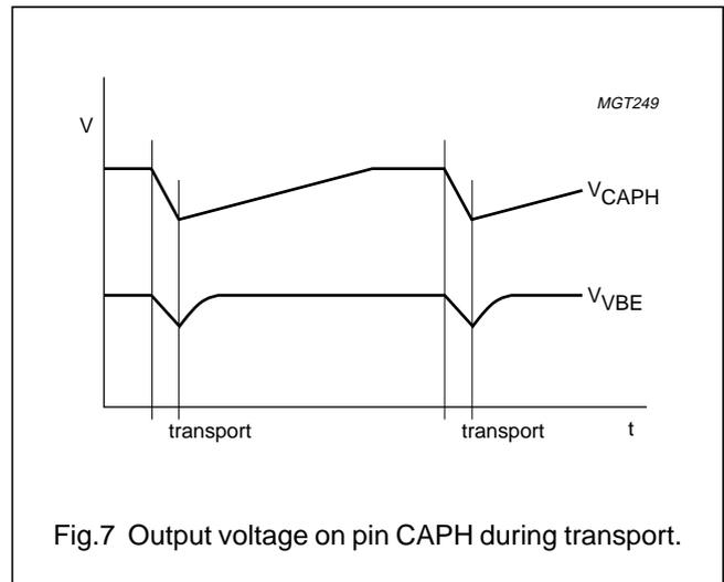
Fig.7 Output voltage on pin CAPH during transport.
