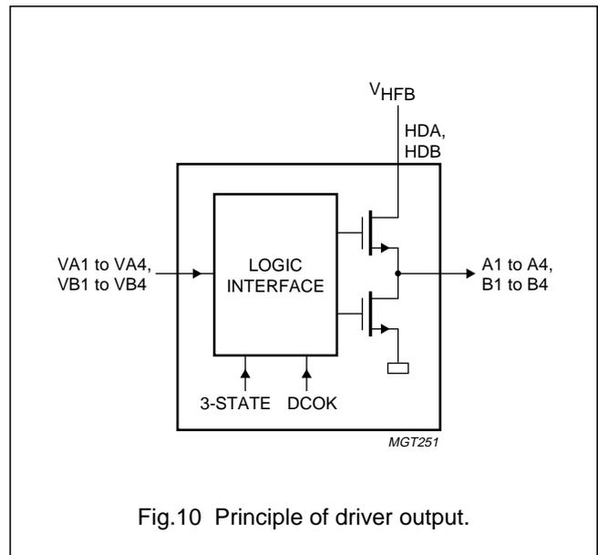
Fig.10 Principle of driver output.
