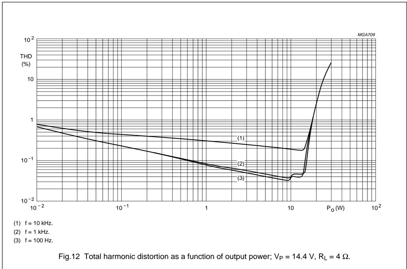
Fig.12 Total harmonic distortion as a function of output power;  $V_P = 14.4 \text{ V}$ ,  $R_L = 4 \Omega$ .
