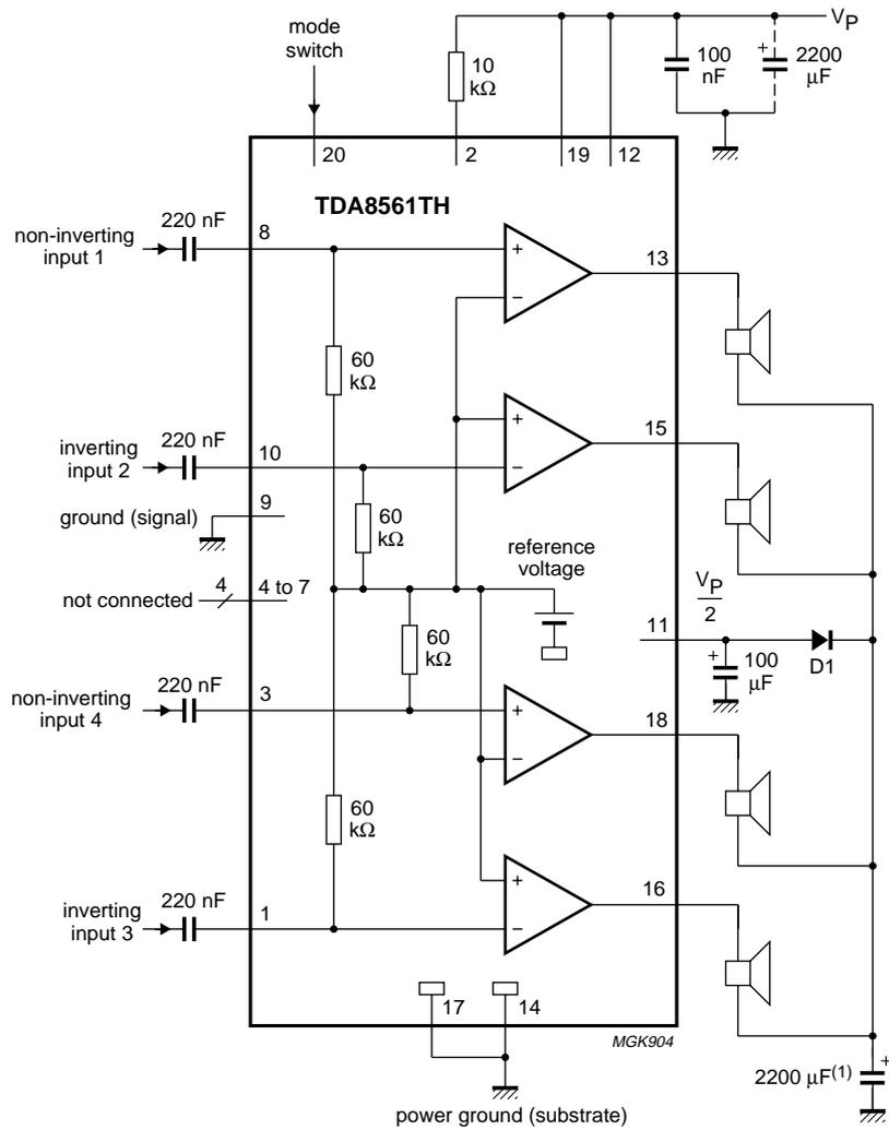
(1) When short-circuiting the single-ended capacitor, the dissipation will be reduced due to diode D1.
