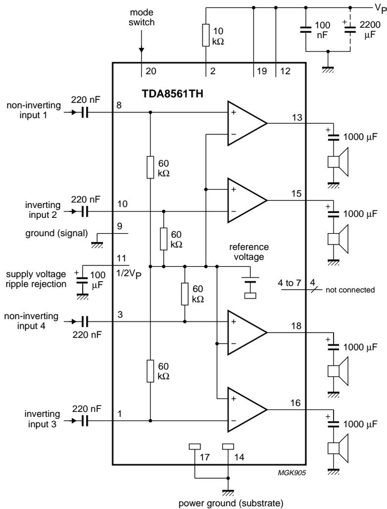
Fig.9 Quad single-ended application diagram 1.
