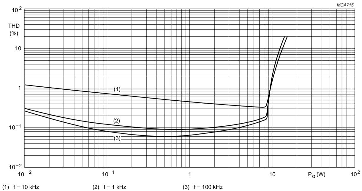
Fig.18 Total harmonic distortion as a function of output power;  $V_P = 14.4$  V,  $R_L = 2 \Omega$ .
