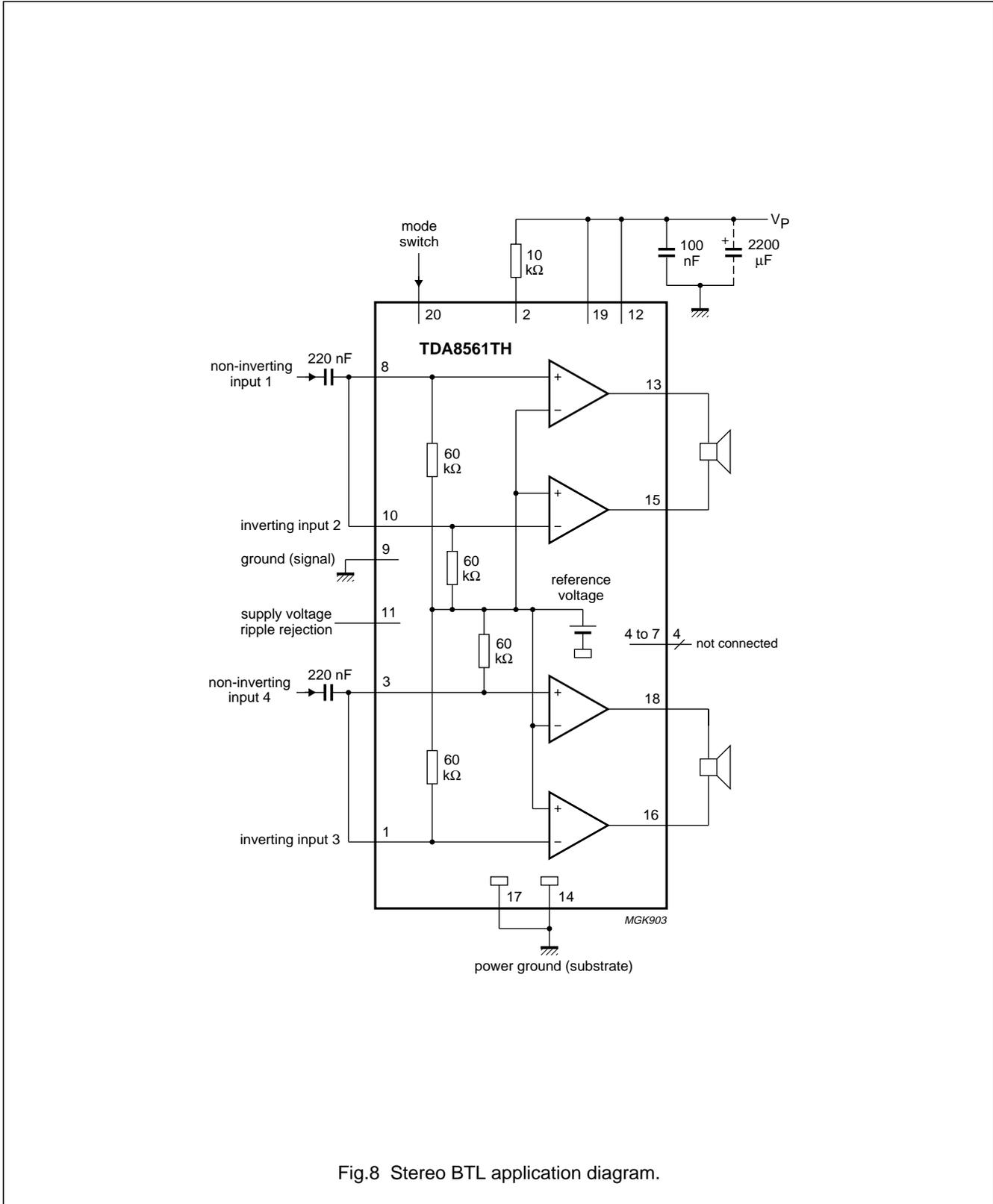
Fig.8 Stereo BTL application diagram.
