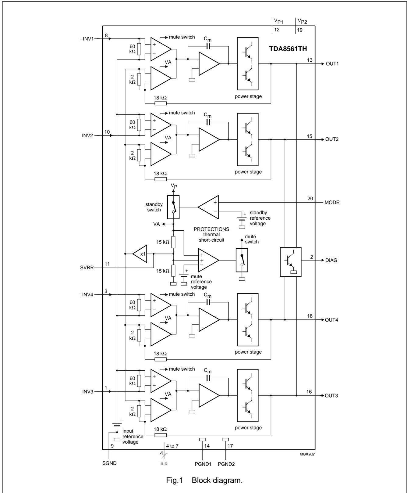
Fig.1 Block diagram.
