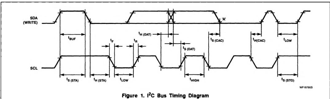
**Figure 1. I<sup>2</sup>C Bus Timing Diagram**
