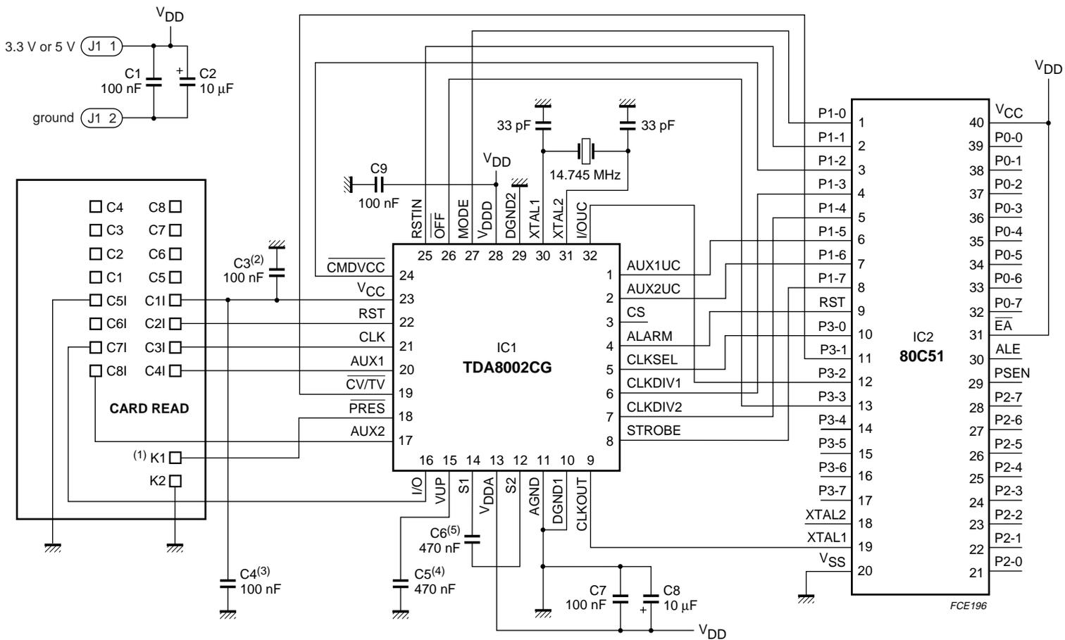
TDA8002C should be placed as close as possible to the card reader.
