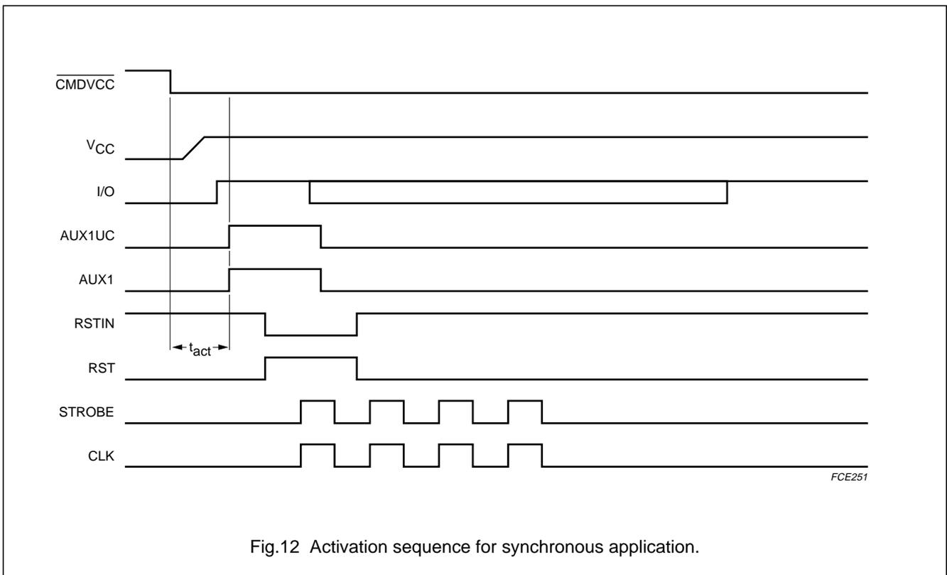
Fig.12 Activation sequence for synchronous application.
