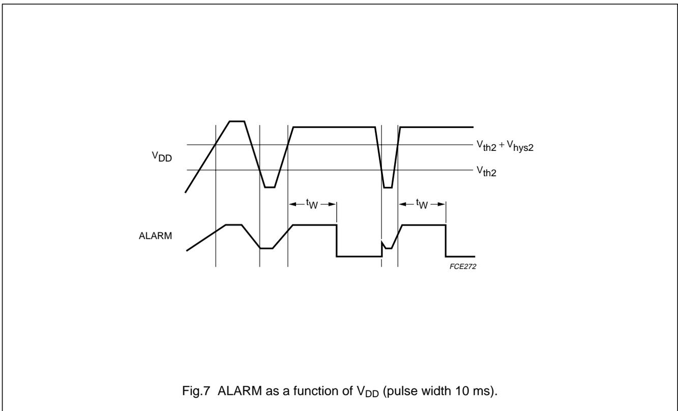
Fig.7 ALARM as a function of  $V_{DD}$  (pulse width 10 ms).
