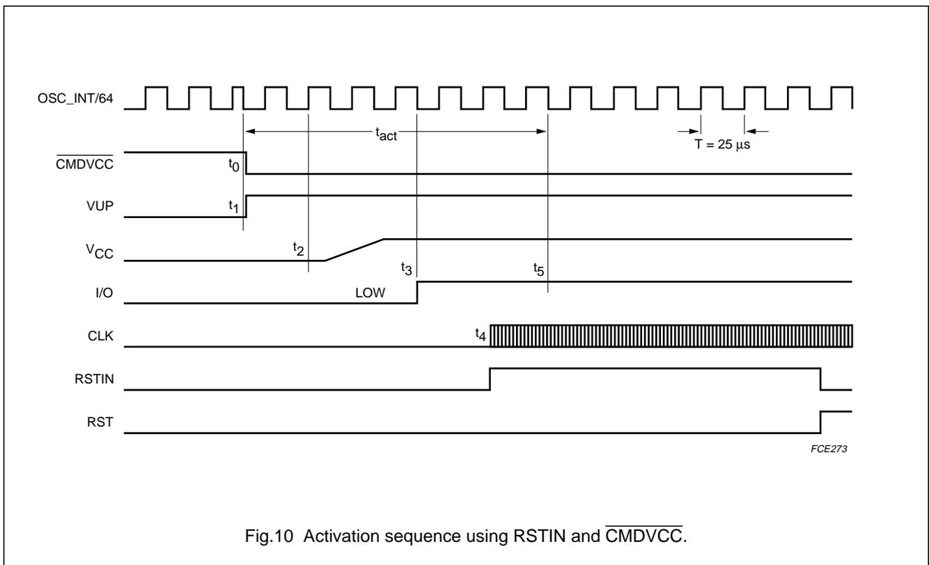
Fig.10 Activation sequence using RSTIN and  $\overline{\text{CMDVCC}}$ .
