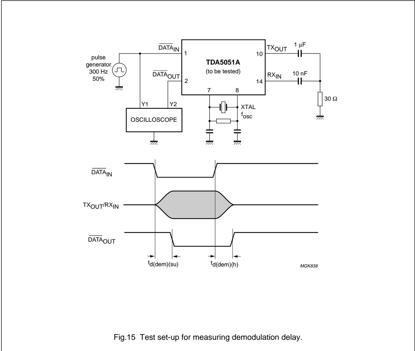
Fig.15 Test set-up for measuring demodulation delay.
