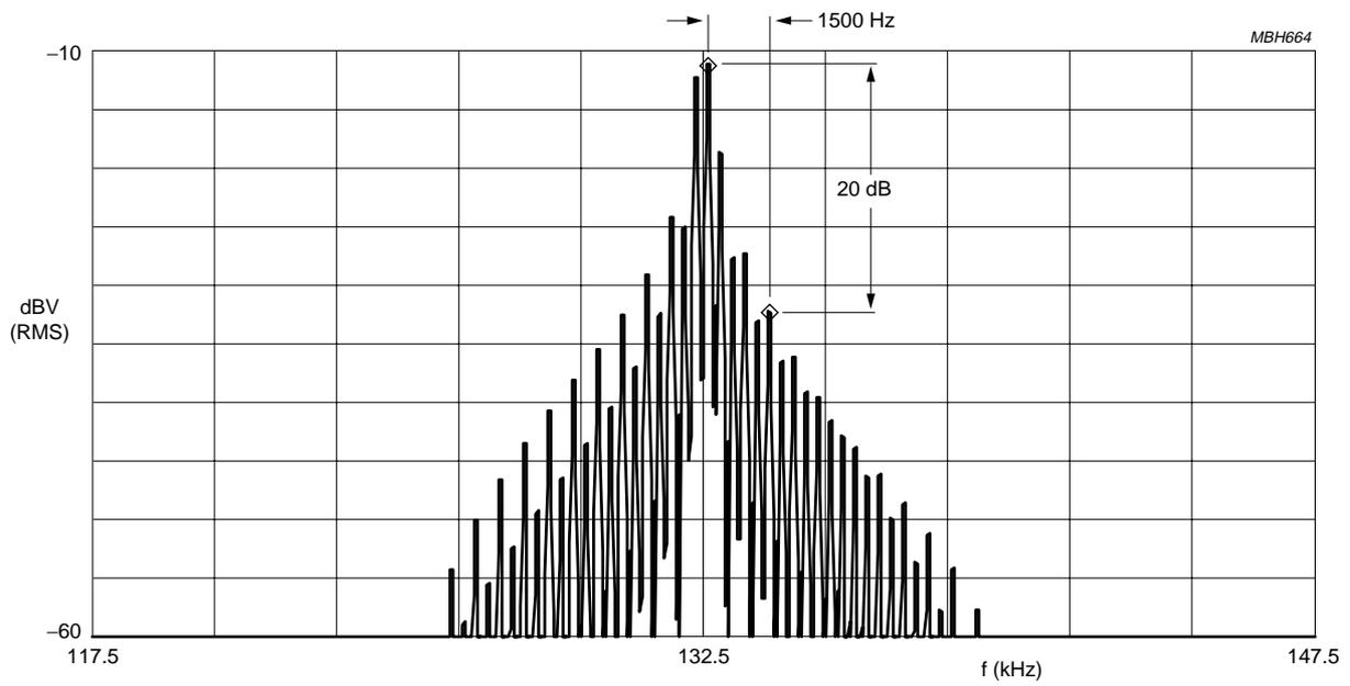
Resolution bandwidth = 100 Hz;  $B_{-20dB} = 3000 \text{ Hz} (2 \times 1500 \text{ Hz})$ .
