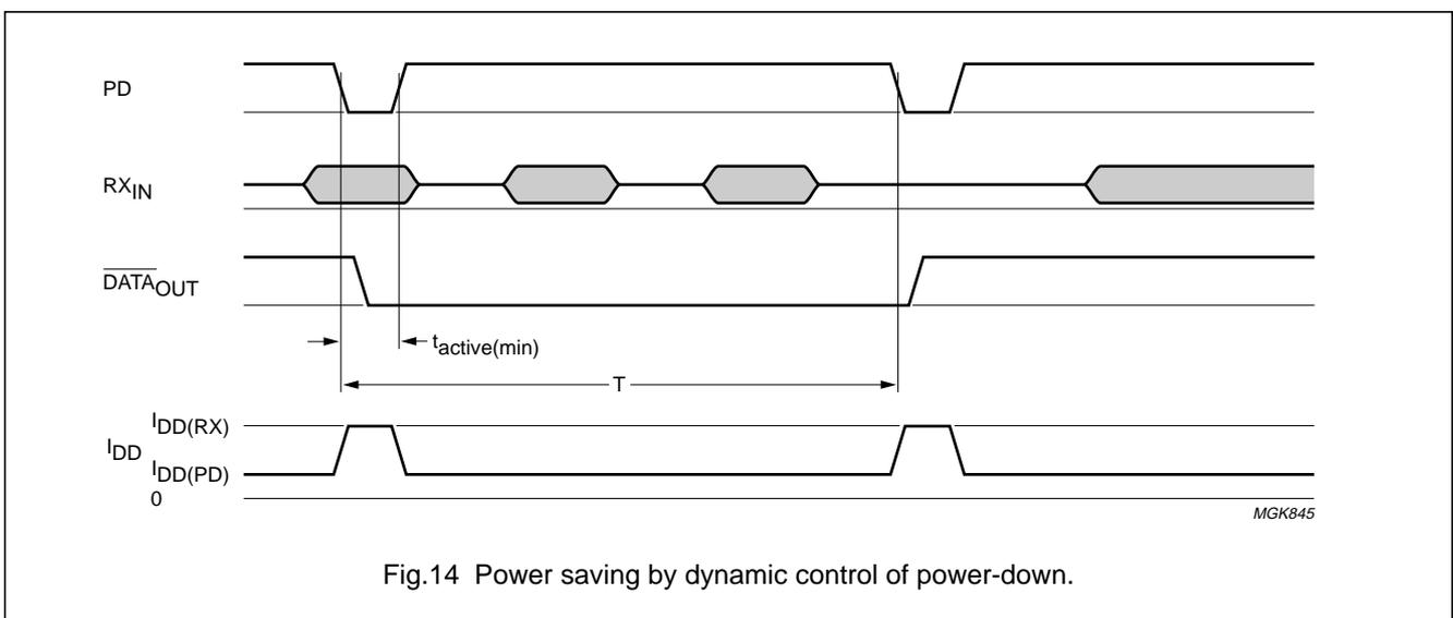
Fig.14 Power saving by dynamic control of power-down.
