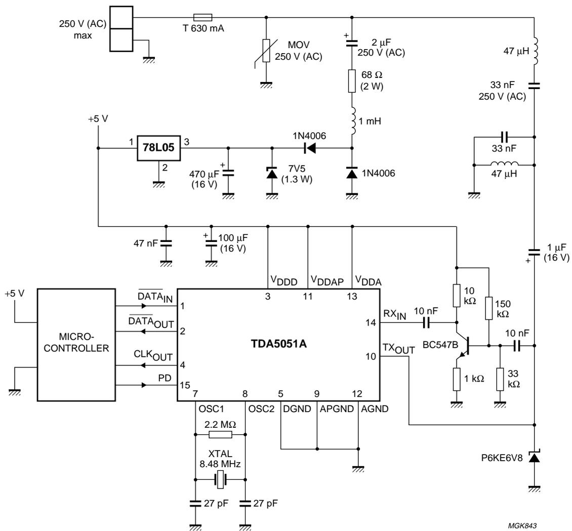
Fig.22 Application diagram without power line insulation, with improved sensitivity.
