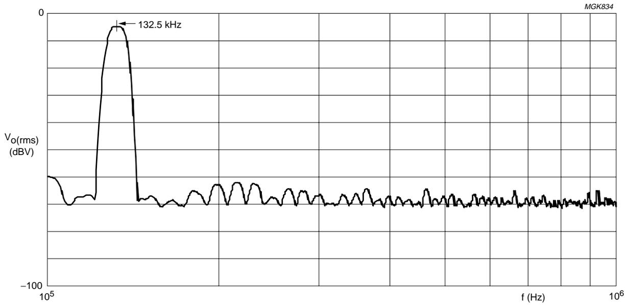
Resolution bandwidth = 9 kHz; top: 0 dBV (RMS) = 120 dB $\mu$ V (RMS); marker at -5 dBV (RMS) = 115 dB $\mu$ V (RMS); the CISPR16 network provides an attenuation of 6 dB, so the signal amplitude is 121 dB $\mu$ V (RMS).
