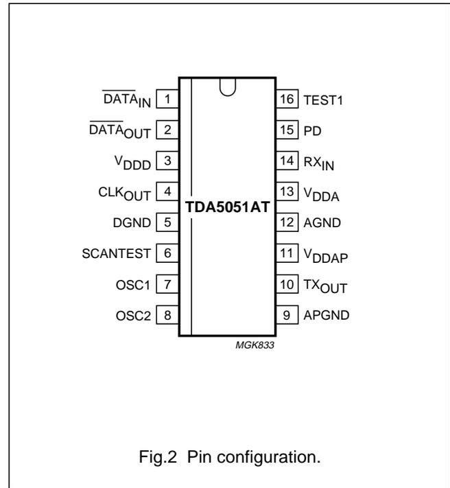
Fig.2 Pin configuration.
