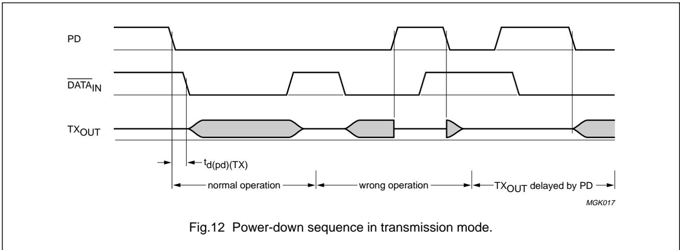
Fig.12 Power-down sequence in transmission mode.
