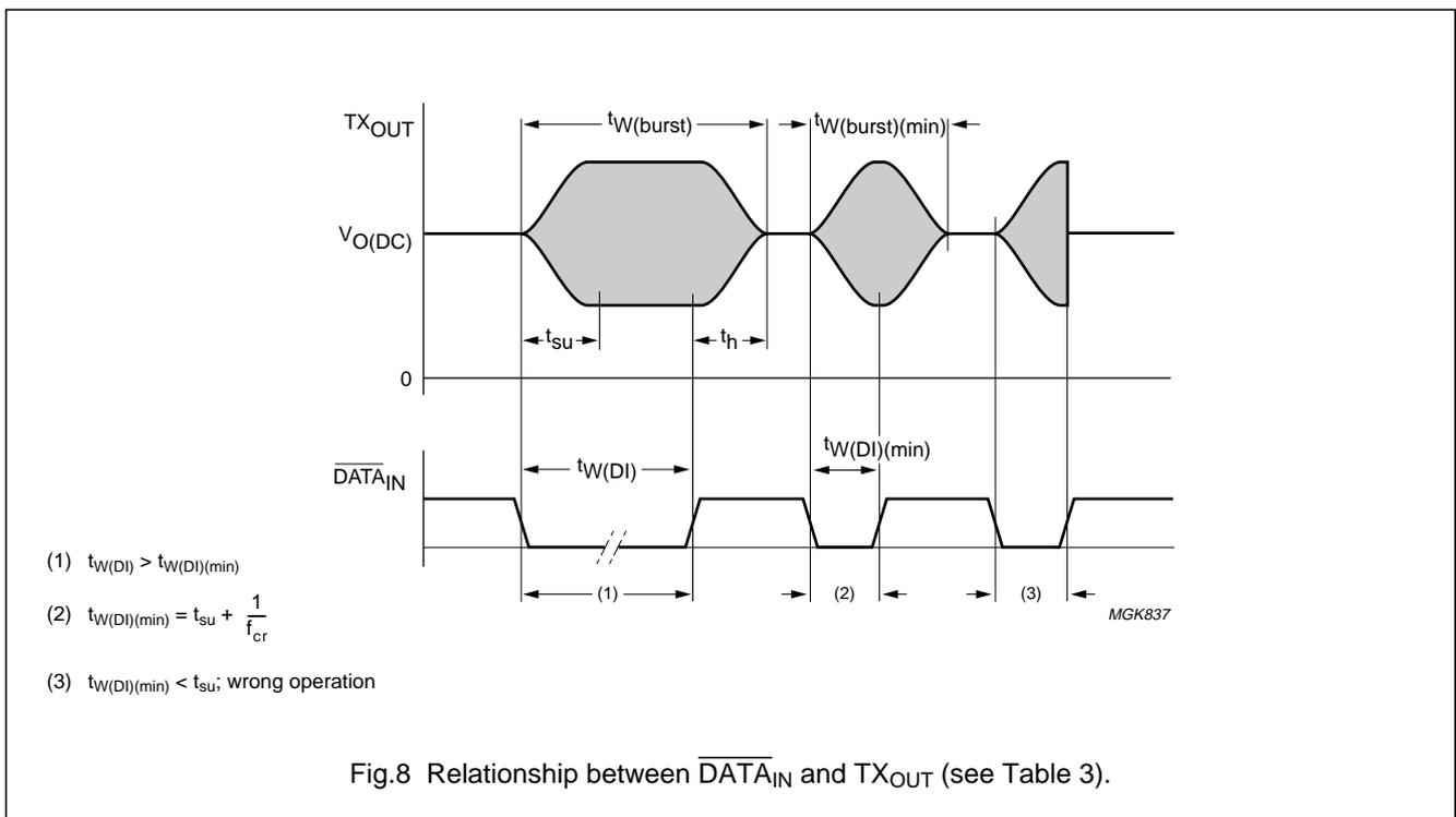
Fig.8 Relationship between  $\overline{DATA}_{IN}$  and  $TX_{OUT}$  (see Table 3).
