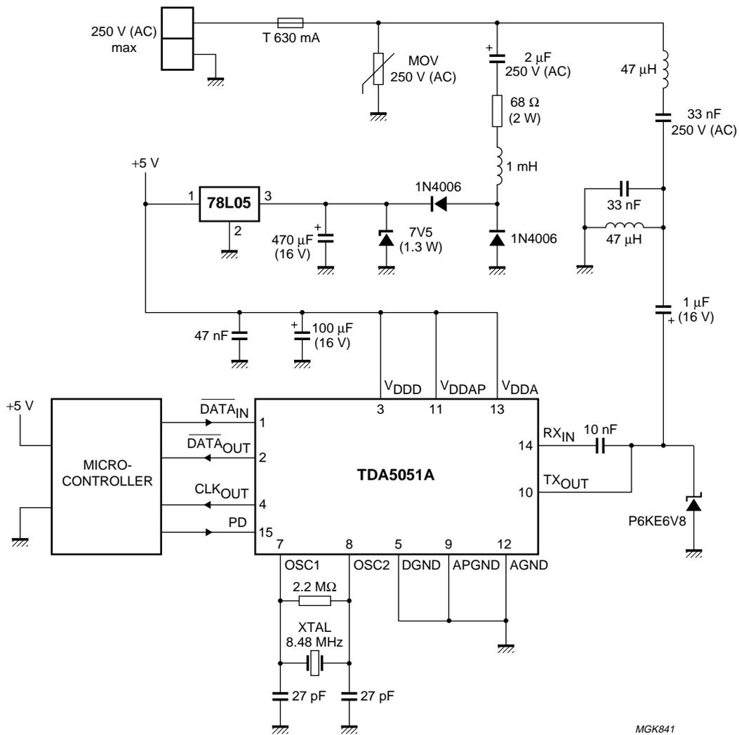
Fig.18 Application diagram without power line insulation.
