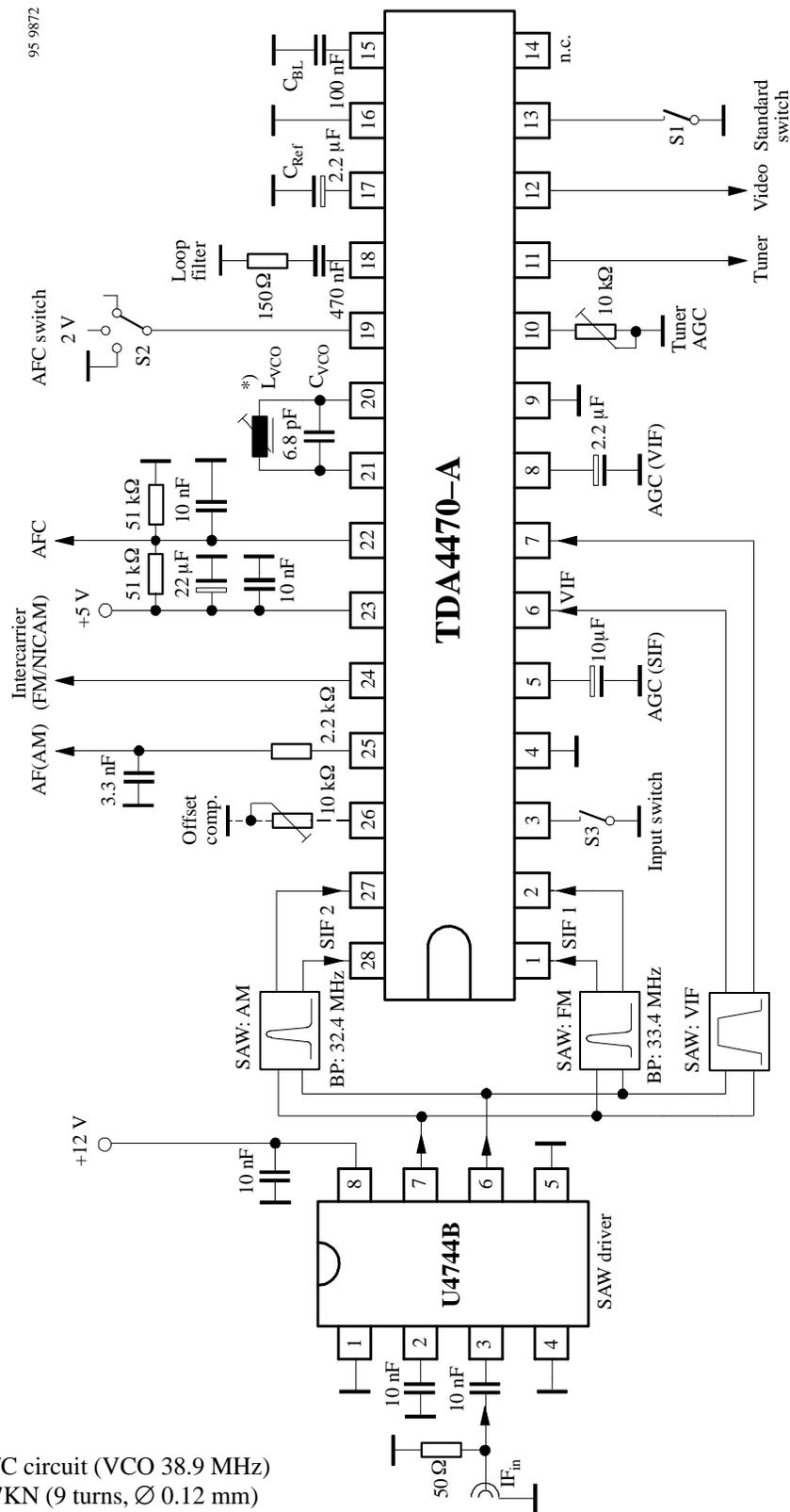
\*) external L/C circuit (VCO 38.9 MHz) with TOKO coil 7KN (9 turns, Ø 0.12 mm)
