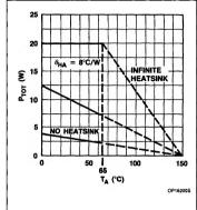
Figure 2. Power Derating Curve
