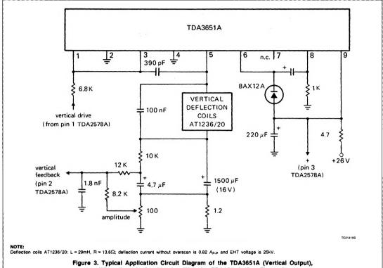
Figure 3. Typical Application Circuit Diagram of the TDA3651A (Vertical Output), When Used in Combination With the TDA2578A (See Figure 5)
