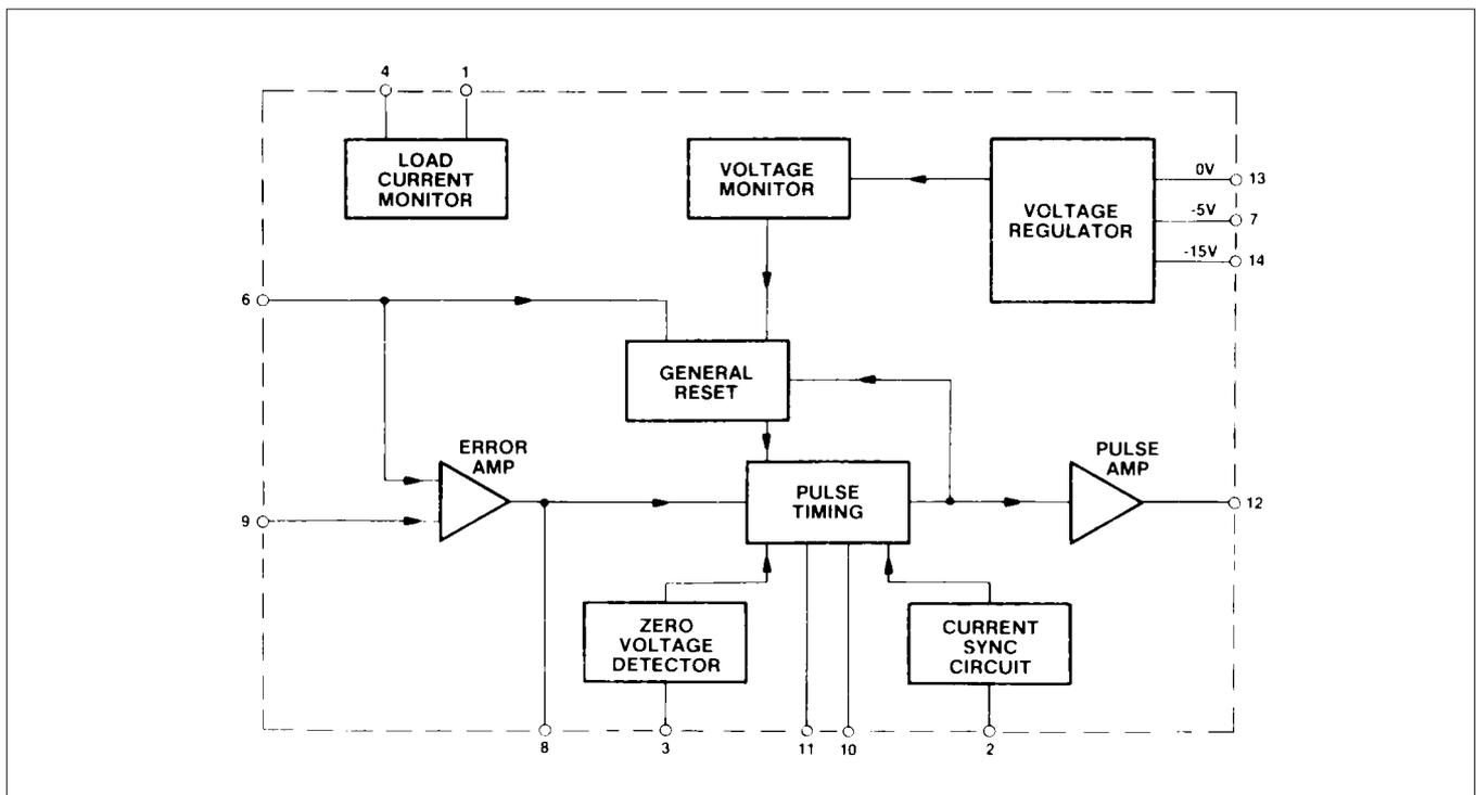
Fig. 2 Block Diagram of TDA2088
