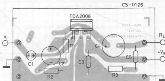
Fig. 3 - 25W bridge configuration application circuit (°)
