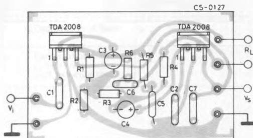
(°) The value of the capacitors C3 and C4 are different to optimize the SVR (Typ. = 40 dB)
