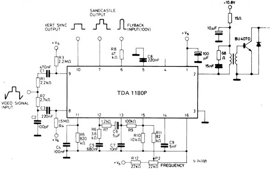
Fig. 9 - Application circuit for Darlington output stage
