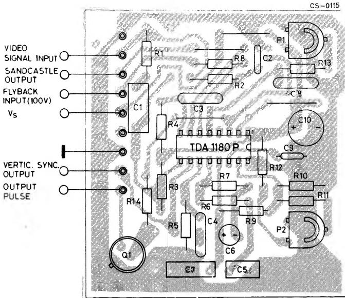
Fig. 8 - Application circuit for small screen b.w. TV.
